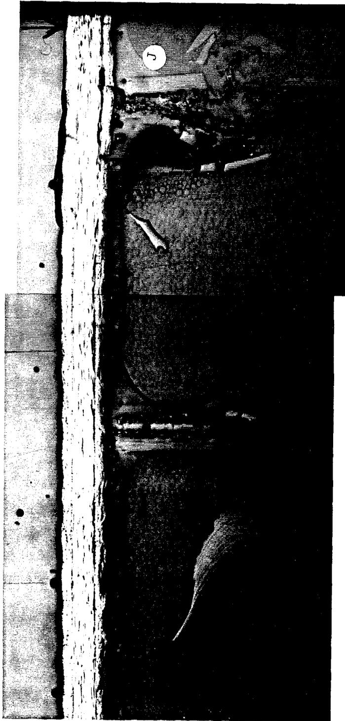
Figure 3.12. 90° Cross-Section 16694-3-2 (25X)
