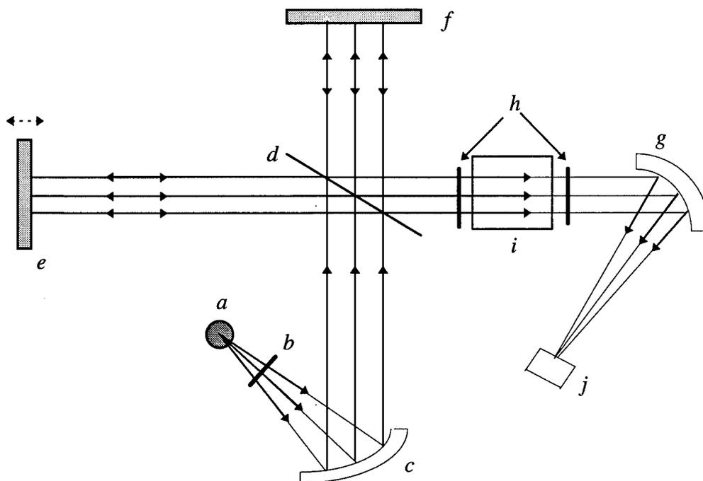
**Figure 3-1.** Michelson Interferometer. *a.* source, *b.* aperture, *c.* collimating mirror, *d.* beamsplitter, *e.* movable mirror, *f.* fixed mirror, *g.* focusing mirror, *h.* spectral filters, *i.* sample cell, and *j.* detector.
