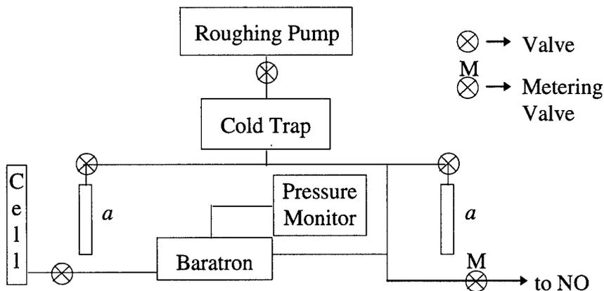
**Figure 3-3.** Vacuum system used to create nitrosyl bromide.
