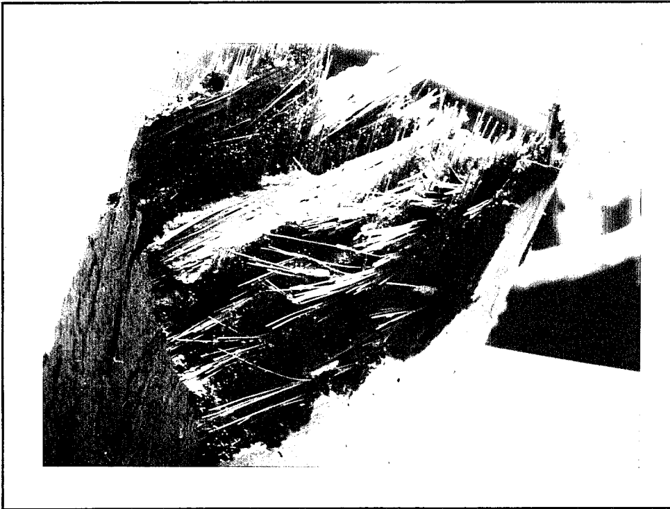
Figure 74. Fracture Surface, Monotonic Tensile, 566 °C, 15.2X
