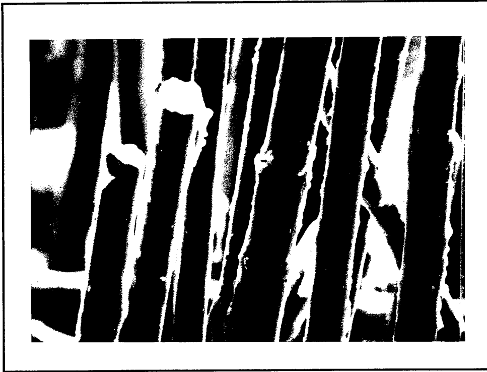
Figure 101. Fiber Surface, 1 Hz, 1093°C, 96.53 MPa, 575X
