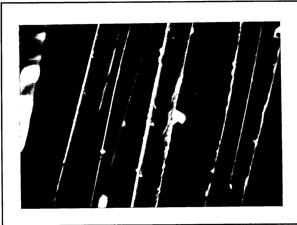
Figure 100. Fiber Surface, 1 Hz, 1093°C, 137.9 MPa, 625X
