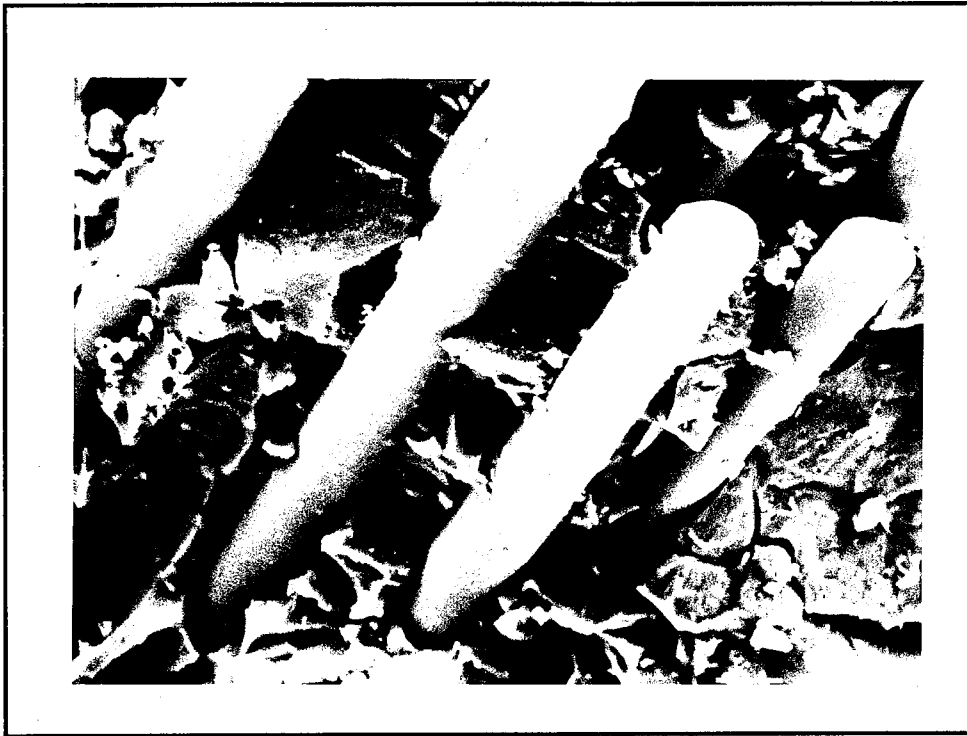
Figure 79. Fiber Surface, 10 Hz, 566°C, 137.9 MPa, 685X
