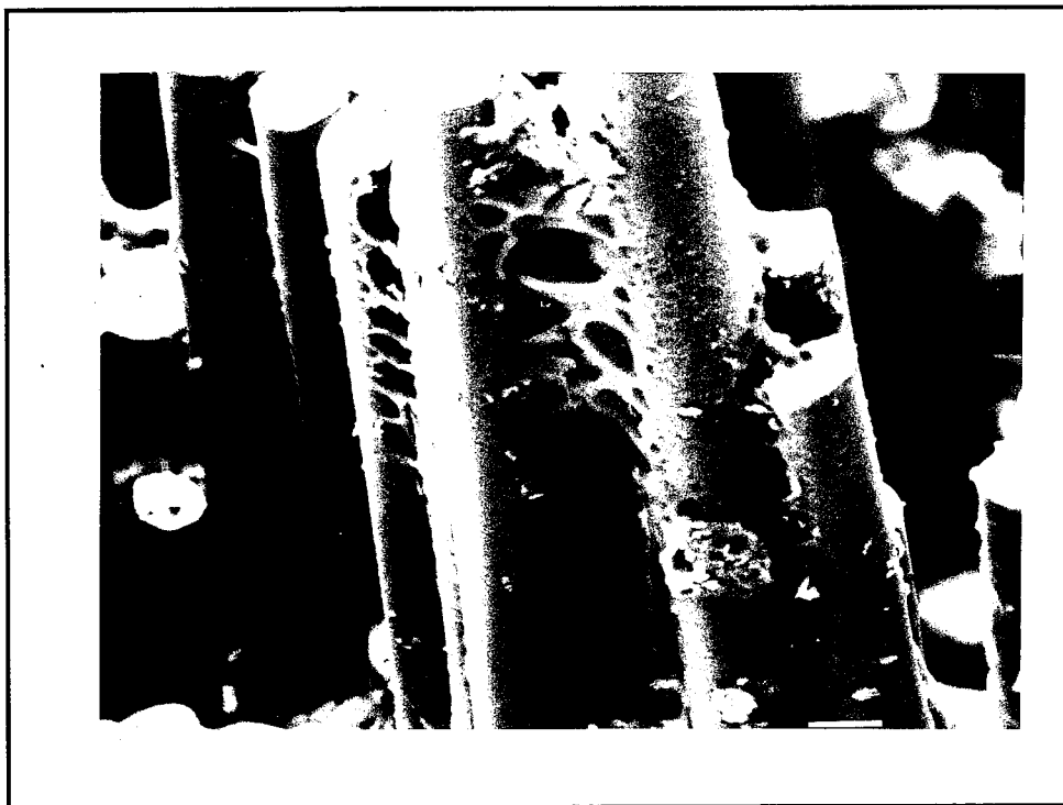
Figure 80. Fiber Surface, 10 Hz, 566°C, 103.43 MPa, 470X
