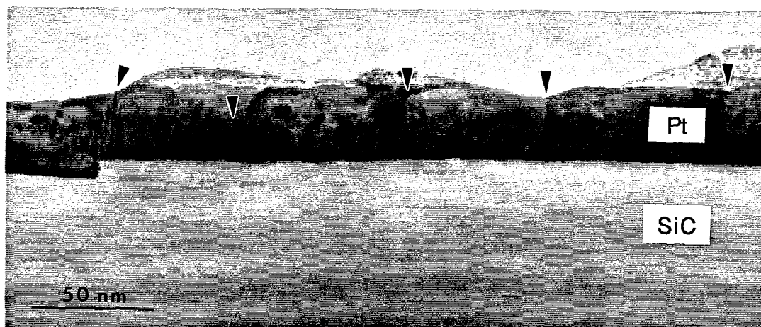
Figure 7. Cross-sectional TEM image of Pt/SiC annealed at 650°C for 20 min. The arrows delineate the grain boundaries. The average grain size of the Pt film was 65 nm.
