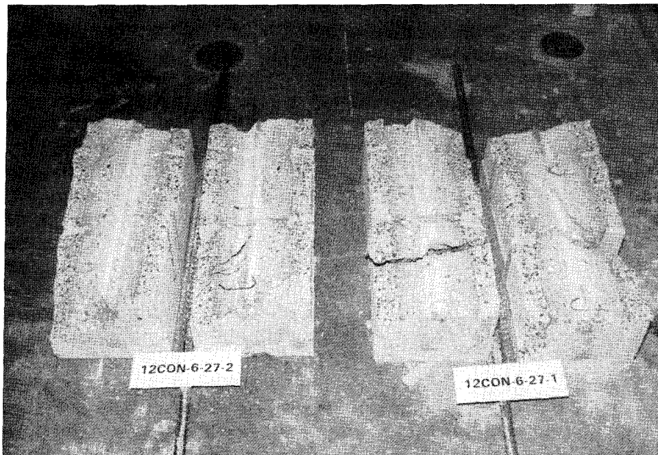
b. Typical splitting failure mode
