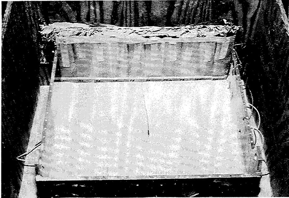
Figure A-21. Soil Pluviated to Sixth Level of Reinforcing
