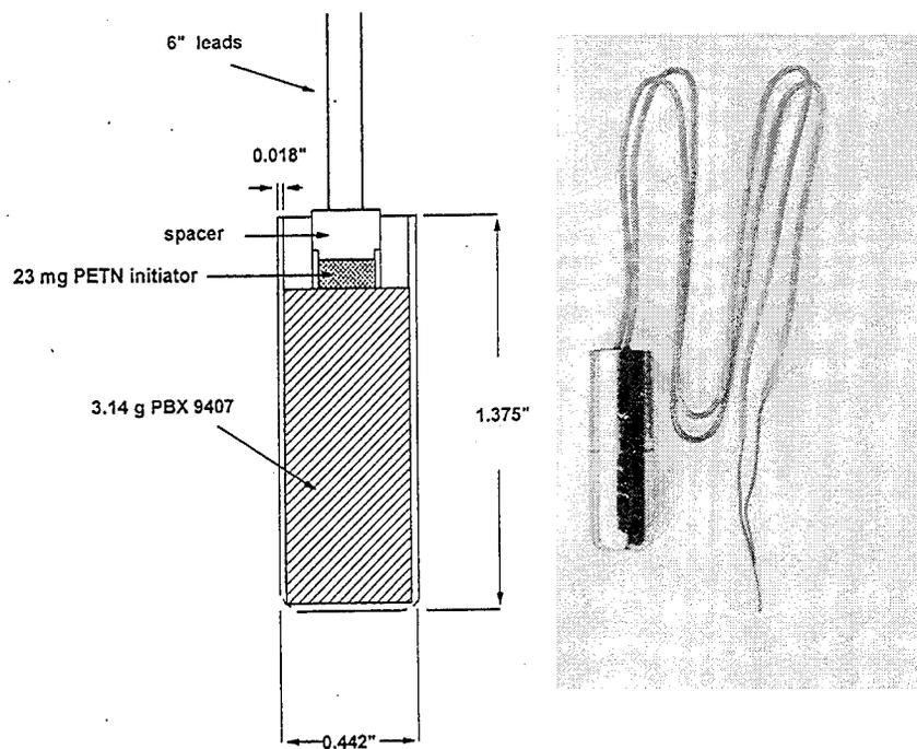
Figure 9. Detonator
