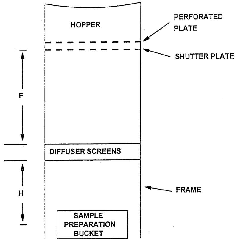
Figure 10. Schematic Diagram: Soil Pluviator
