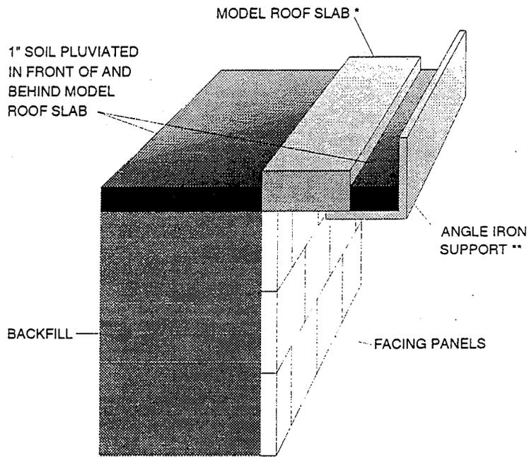
\* MODEL ROOF SLAB MASS IS EQUAL TO MASS OF ROOF SLAB PLUS MASS OF 2.5 FOOT-THICK SOIL OVERBURDEN.
