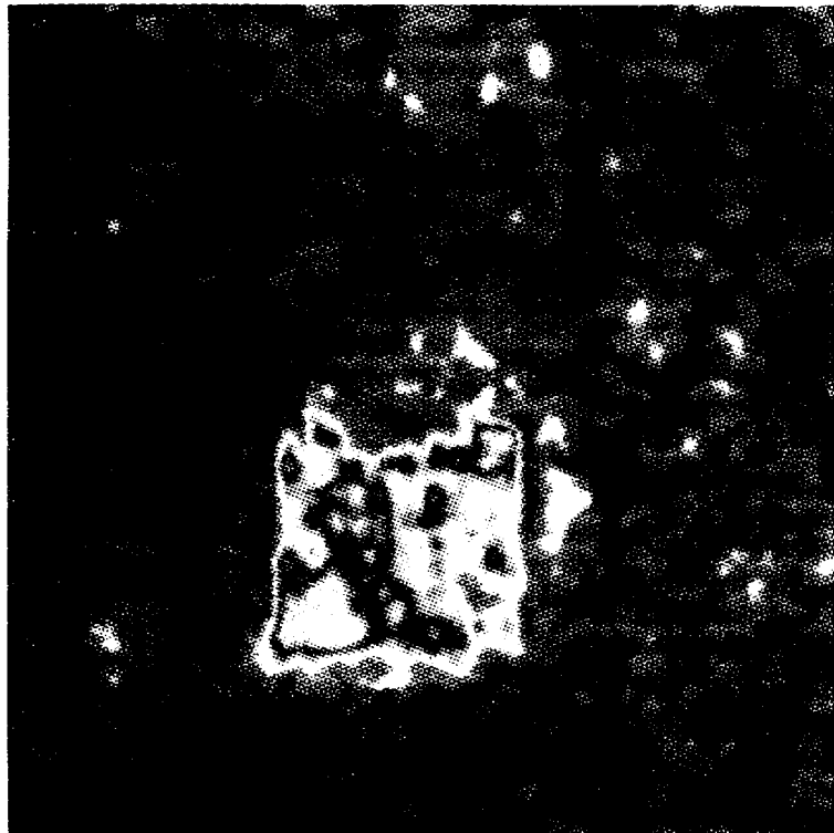
Figure 1. Ultrasonic image of a thick composite panel with simulated damage.
