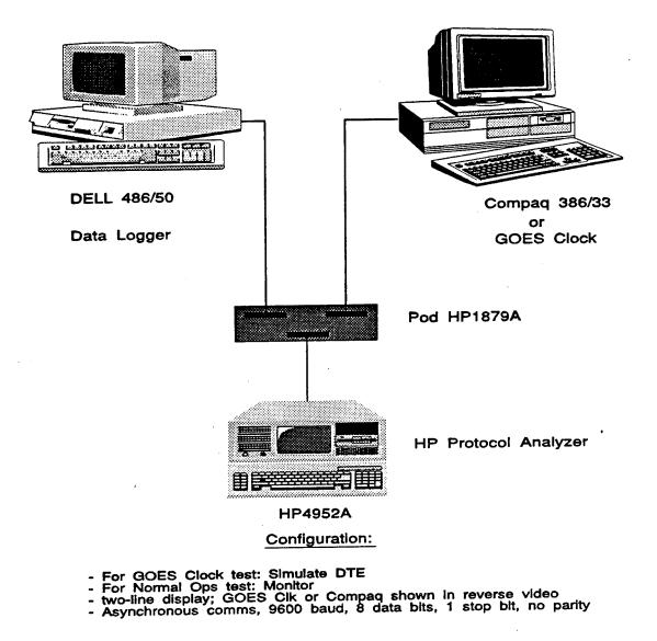
Fig. 7.1 Hookup Schematic for Testing Procedures
