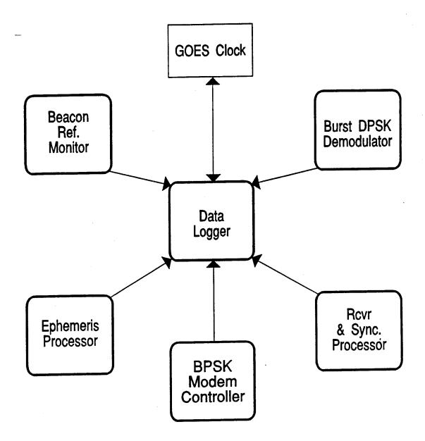
Fig. 2.2 Interconnecting Diagram between Data Logger and Other Processors
