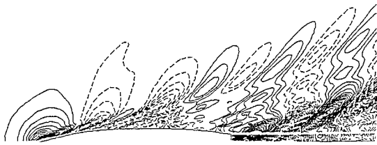
Fig. 16 — Contours of the computed free-surface elevation for Model 5415 at F = 0.25 . Solid lines indicate positive wave elevation Z/F^2 = 0.005j for j = 1, 2, \text{etc.} , and dashed lines, negative wave elevation Z/F^2 = -0.005j for j = 1, 2, \text{etc.} The zero contour is not drawn.
