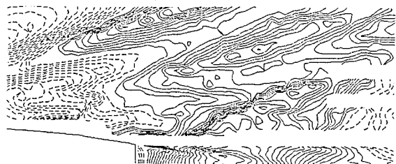
Fig. 14 — Contours of the free-surface elevation near the transom stern of Model 5415 at F = 0.414 . (a) Contours of computed wave elevation. (b) Contours of measured wave elevation except aft of the transom where contours of computed wave elevation are presented (and are identical to the corresponding contours in (a)). Contour levels are the same as in Fig. 13
