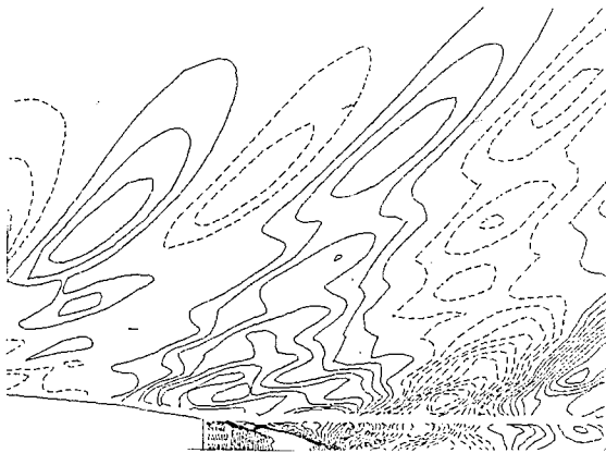
Fig. 19 — Contours of computed free-surface elevation for Model 5415 hull at F = 0.25 . Paneling behind the transom stern has been placed on the mean free-surface level. Finite differencing at the upstream end of strips of panels originating at the stern involves the disturbance potential only at the centroids of free-surface panels instead of at the centroids of neighboring free surface and hull panels. Solid lines indicate positive wave elevation Z/F^2 = 0.005j for j = 1, 2 , etc. and dashed lines, negative elevation Z/F^2 = -0.005j for j = 1, 2 , etc. The zero contour level has not been drawn.
