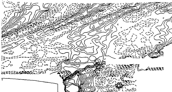
Fig. 17 — Contours of the free-surface elevation near the stern of Model 5415 at F = 0.25 . (a) Contours of computed wave elevation. (b) Contours of measured wave elevation. Contour levels are the same as in Fig. 16.
