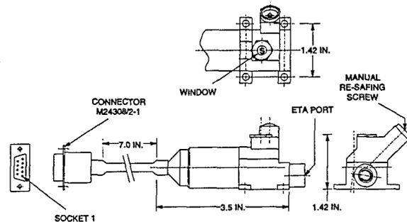
**Figure 4. Safe-and-Arm Device**
