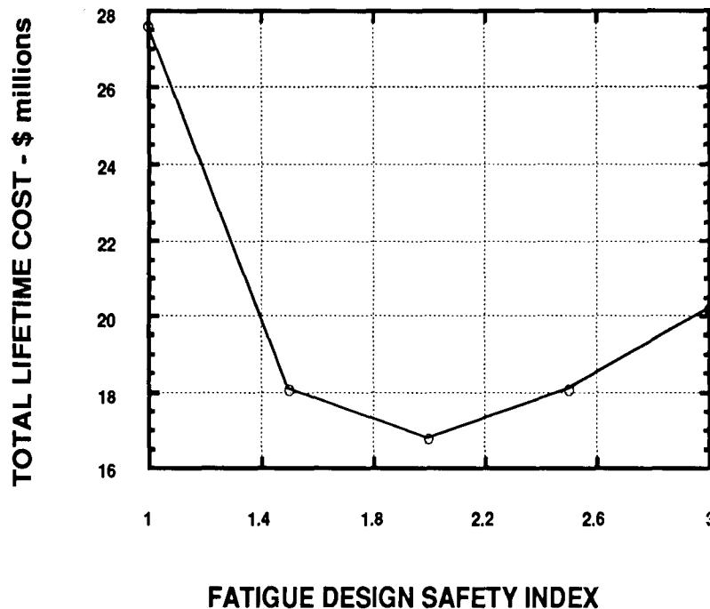
Figure 4.7 - Lifetime (20 year) costs in example ULCC hull structure as function of the fatigue design safety index
