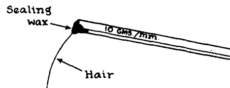
FIGURE 108.—Graduated hair after von Frey for measuring threshold of sensibility to touch (superficial pressure).
