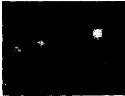
Fig.5 Dark field TEM image of BST film deposited at 600 °C.
