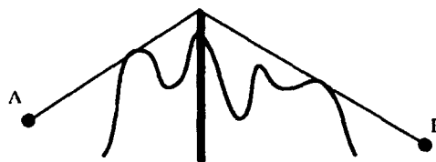
Figure 4. A complex obstacle (the irregular curve) and a Bullington equivalent knife edge (the thick vertical line).
