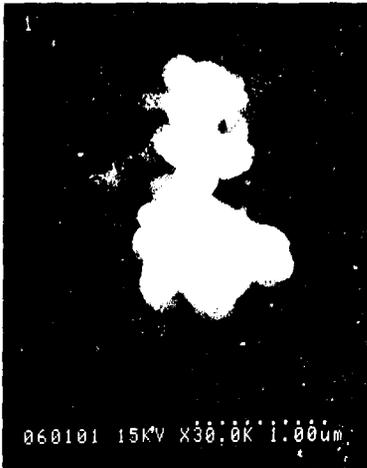
**Figure 6.** A scanning electron microscopy micrograph of an agglomerated particle wafer contaminate produced at low power in the GEC reference cell.
