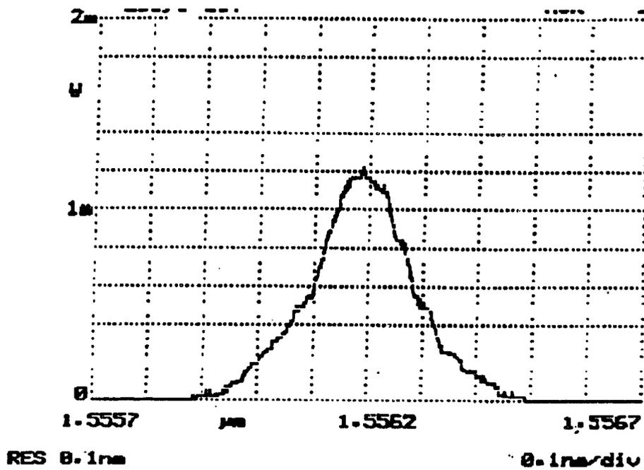
Fig. 12. Optical spectrum of pulse shown in Fig. 4
