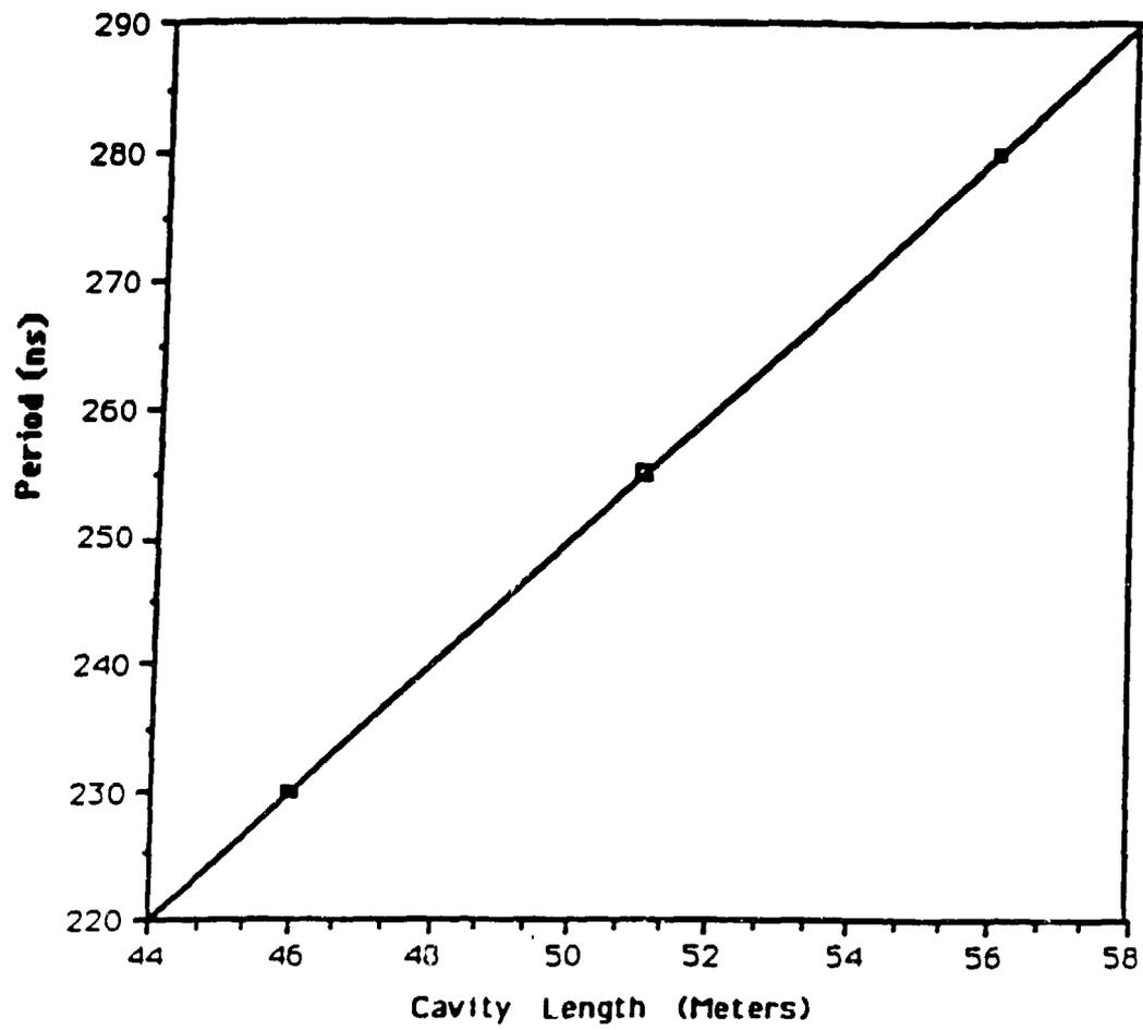
Fig. 7 Period of output pulses as a function of cavity length.
