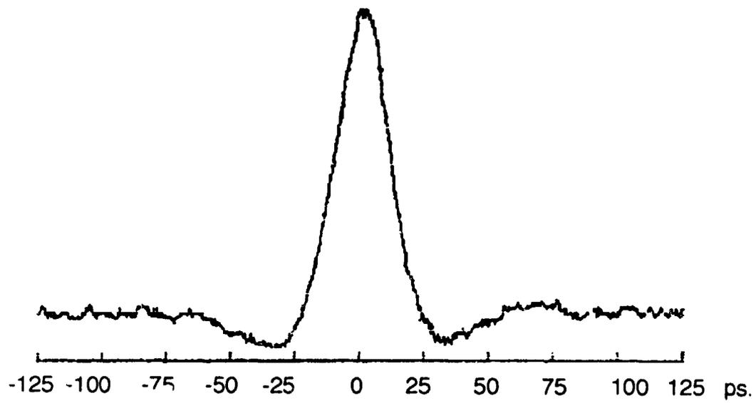
Fig.10 Autocorrelation trace of output pulses with polarizing isolator at a pump power of 50 mW.
