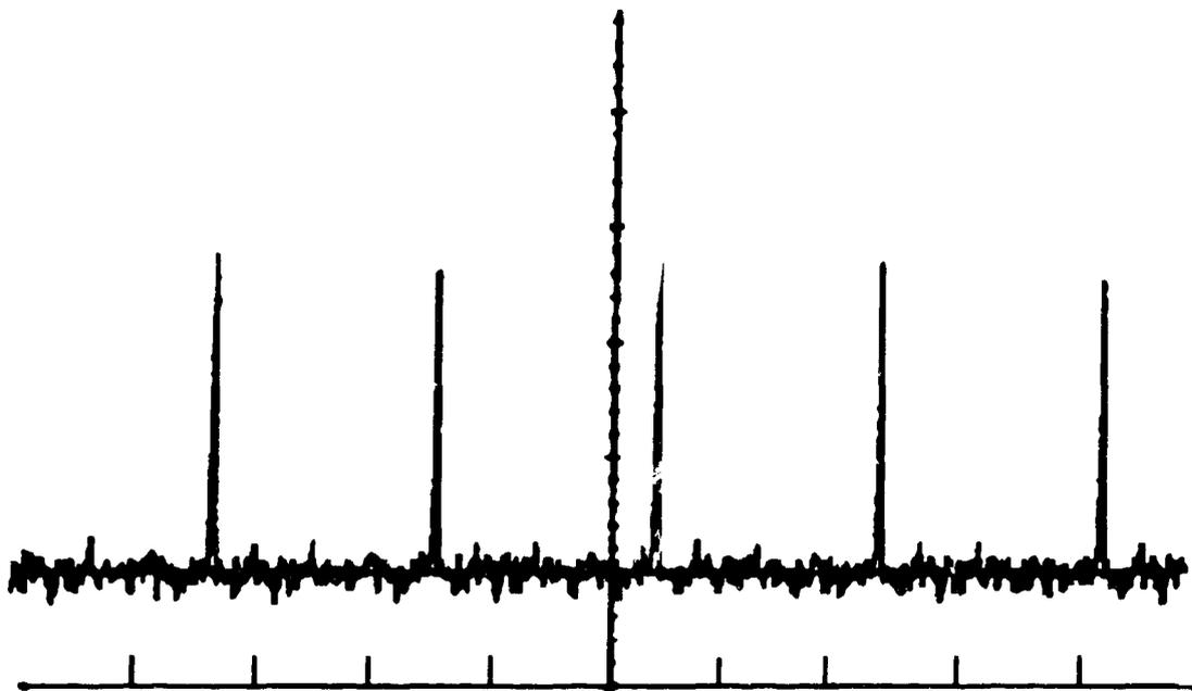
Fig. 9. Mode-locked pulse train. One division equals 50 ns. The period of the pulses was 189 ns.
