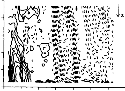
Fig. 9 (b). Contours of Reynolds shear stress. Dashed contours range from -9 to -1 (\text{mm/s})^2 , solid contours 1 to 9 (\text{mm/s})^2 .
