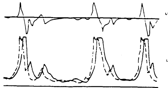
Figure 4 Signal fluctuations and differencing for a 100 micron coal particle
