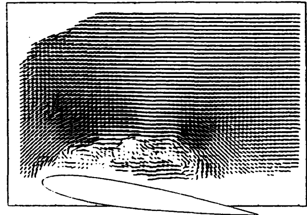
Fig. 2. Instantaneous flow field above NACA 0012 airfoil at \alpha = 24^\circ in upstroke motion and U_\infty = 28 \text{ m/s} ; U_{\text{shift}} = 128 \text{ m/s} .
