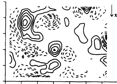
Fig. 11 (a). Instantaneous vorticity contours. Dashed contours range from -4 to -0.5 \text{s}^{-1} , solid contours 0.5 to 4 \text{s}^{-1} . Contour level interval 0.5 \text{s}^{-1} .
