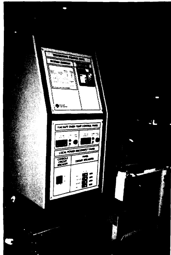
Figure 23. Heater Box With Control Unit Used For Aluminum Doubler Bonding
