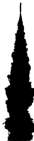
Figure 3. All source fluid is contained within a half angle of 12^\circ . The experiment used Potassium Permanganate. Re = 3,225 .
