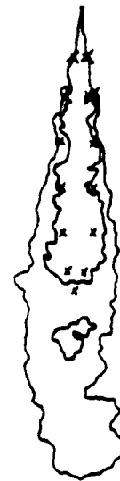
Figure 5. Tracing for Re = 3,225 . Everything above 4.26% is visible. The dark zone is contained within the lighter zone. X's mark the zone given by Eq.(5).
