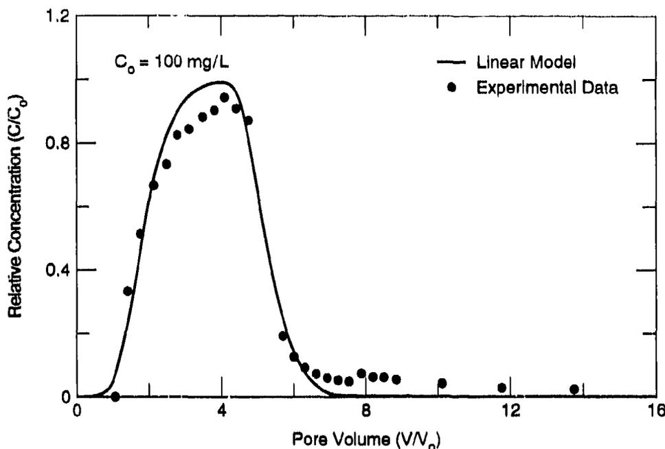
Figure 8. TNT breakthrough results (closed circles) for a bentonite-sand column with input TNT concentration ( $C_0$ ) of 100  $\mu\text{g/mL}$  in a 50% methanol background solution. The solid curve is a model prediction using the transport equation with a linear retention model.
