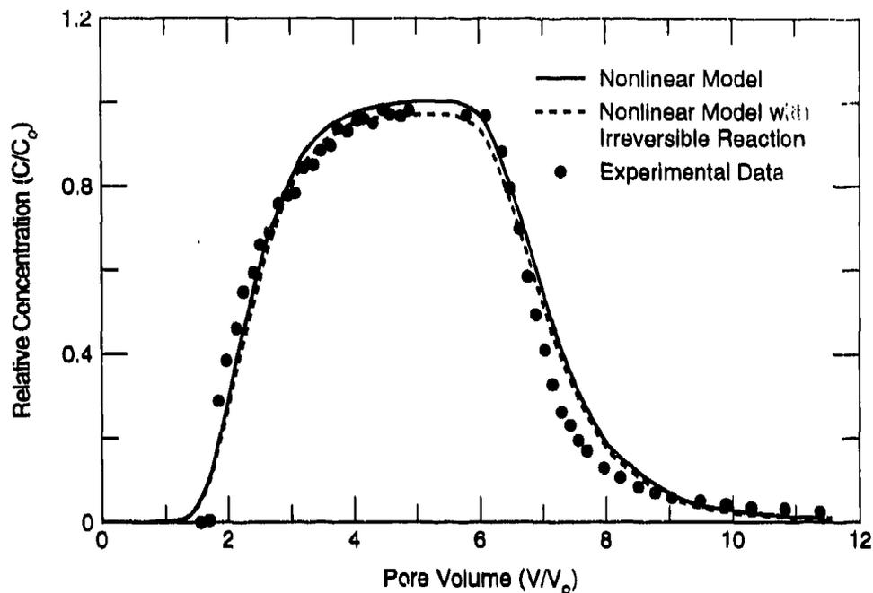
Figure 11. RDX breakthrough results (closed circles) for Kolin uncontaminated soil column with input RDX concentration ( $C_0$ ) of  $10.04 \mu\text{g/mL}$  in  $0.005\text{-M Ca(NO}_3)_2$ . The solid curve is calculated using the transport equation with nonlinear retention whereas the dashed curve includes irreversible reaction.
