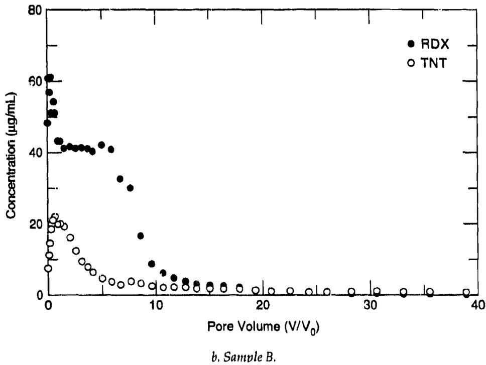
Figure 14. TNT and RDX breakthrough results (pore volume,  $V/V_0$ , vs. relative concentration,  $C/C_0$ ) for the contaminated soil samples obtained from the Louisiana Army Ammunition Plant. The input solution was 0.005-M  $\text{Ca}(\text{NO}_3)_2$ .
