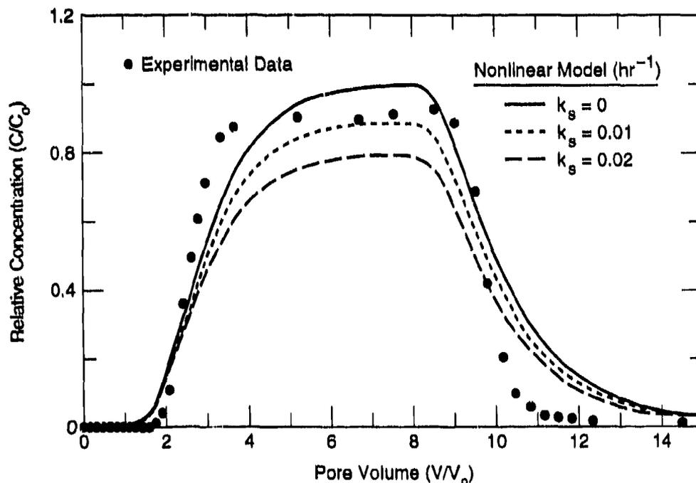
Figure 10. RDX breakthrough results (closed circles) for a bentonite-sand column with input RDX concentration ( $C_0$ ) of 10.65  $\mu\text{g}/\text{mL}$  in a 0.005-M  $\text{Ca}(\text{NO}_3)_2$  background solution. The curves are calculations using the transport equation with nonlinear equilibrium retention and an irreversible reaction for  $k_s$  of 0, 0.01 and 0.02 hr<sup>-1</sup>.
