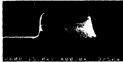
Fig. 4: SEM micrograph of a cleaved Si mesa. Mask aperture oriented along \langle 100 \rangle . Growth temperature: 500^\circ\text{C} , growth rate: 0.27\ \text{nm/s} .
