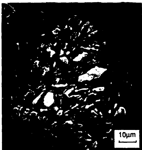
Figure 1: Back-scattered electron image of the powder mixture after 24 hours of ball milling.
