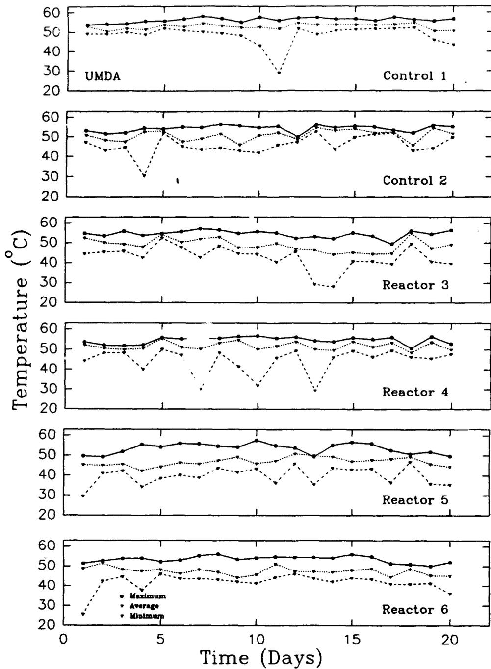
Figure 21. Mean daily maximum, average, and minimum temperatures in composted Umatilla reactors from Experiment VI. Each datum point represents average of 30-min readings recorded in each 24-hr period. Controls received no radiolabeled TNT
