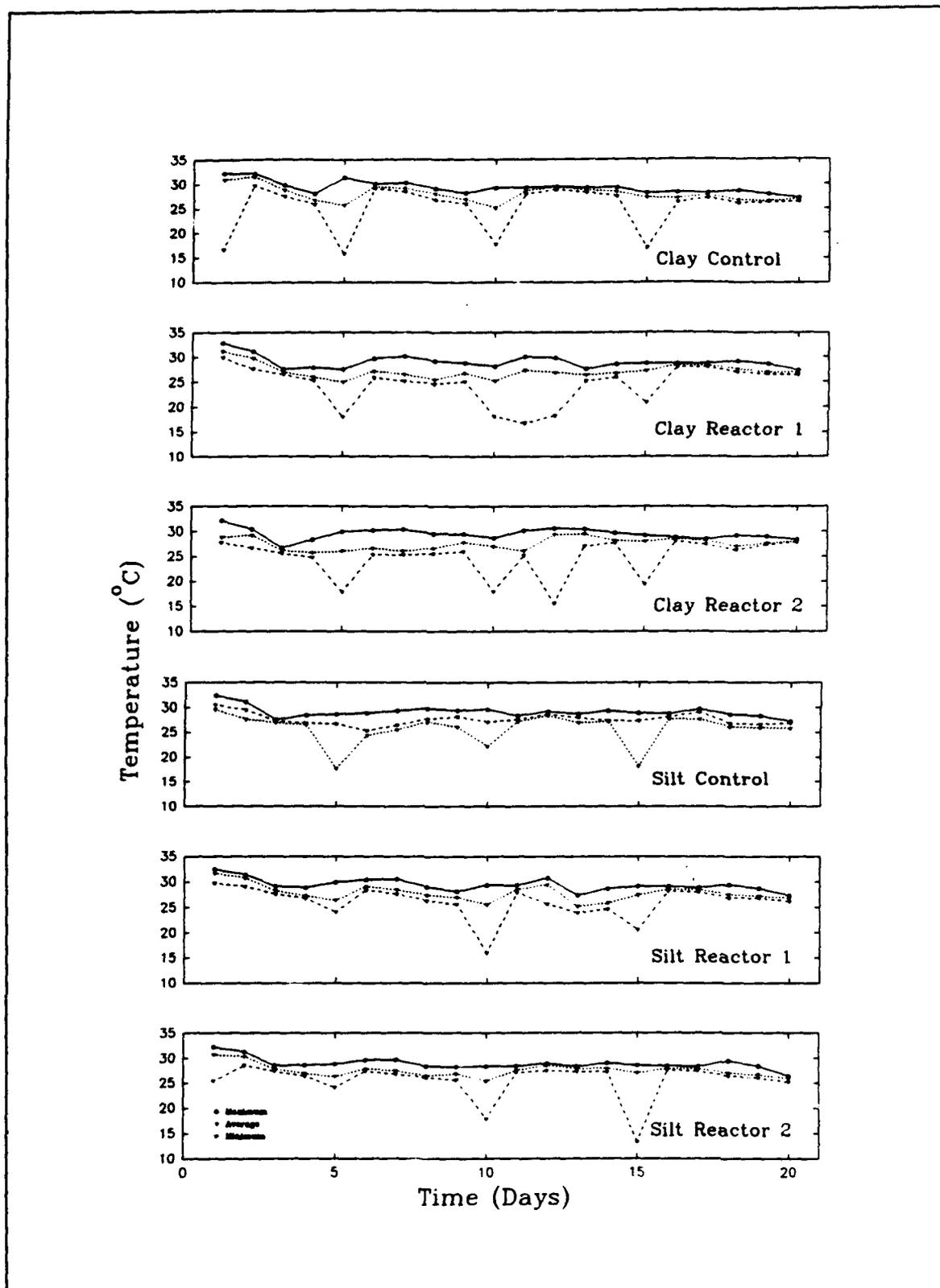
Figure 6. Mean daily maximum, average, and minimum temperatures in composted clay and silt reactors from Experiment 1. Each datum point represents average of all 30-min readings recorded in each 24-hr period. Controls received no TNT
