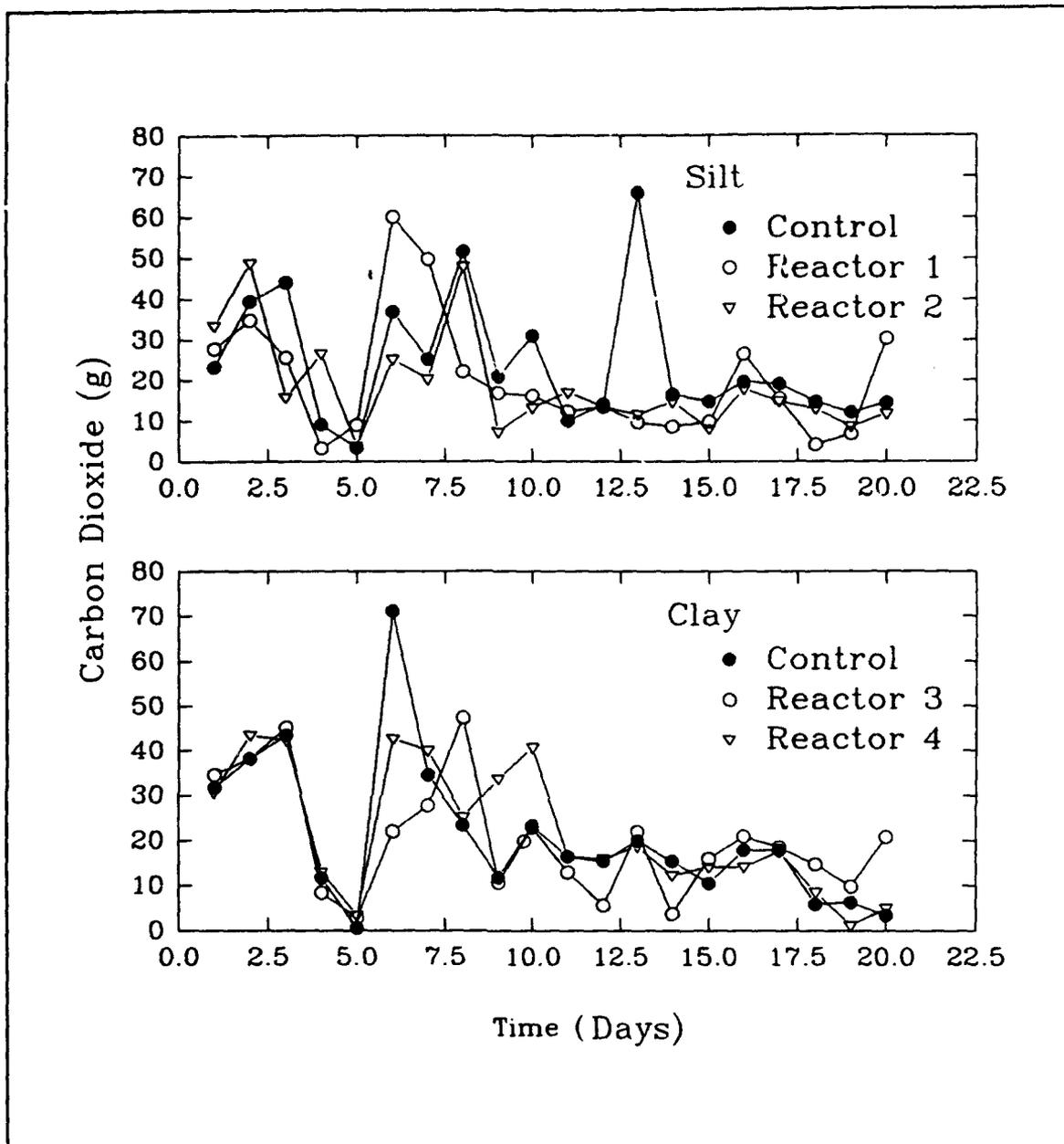
Figure 14. Daily total carbon dioxide evolved from each reactor from Experiment IV. Each datum point represents sum of two traps in series
