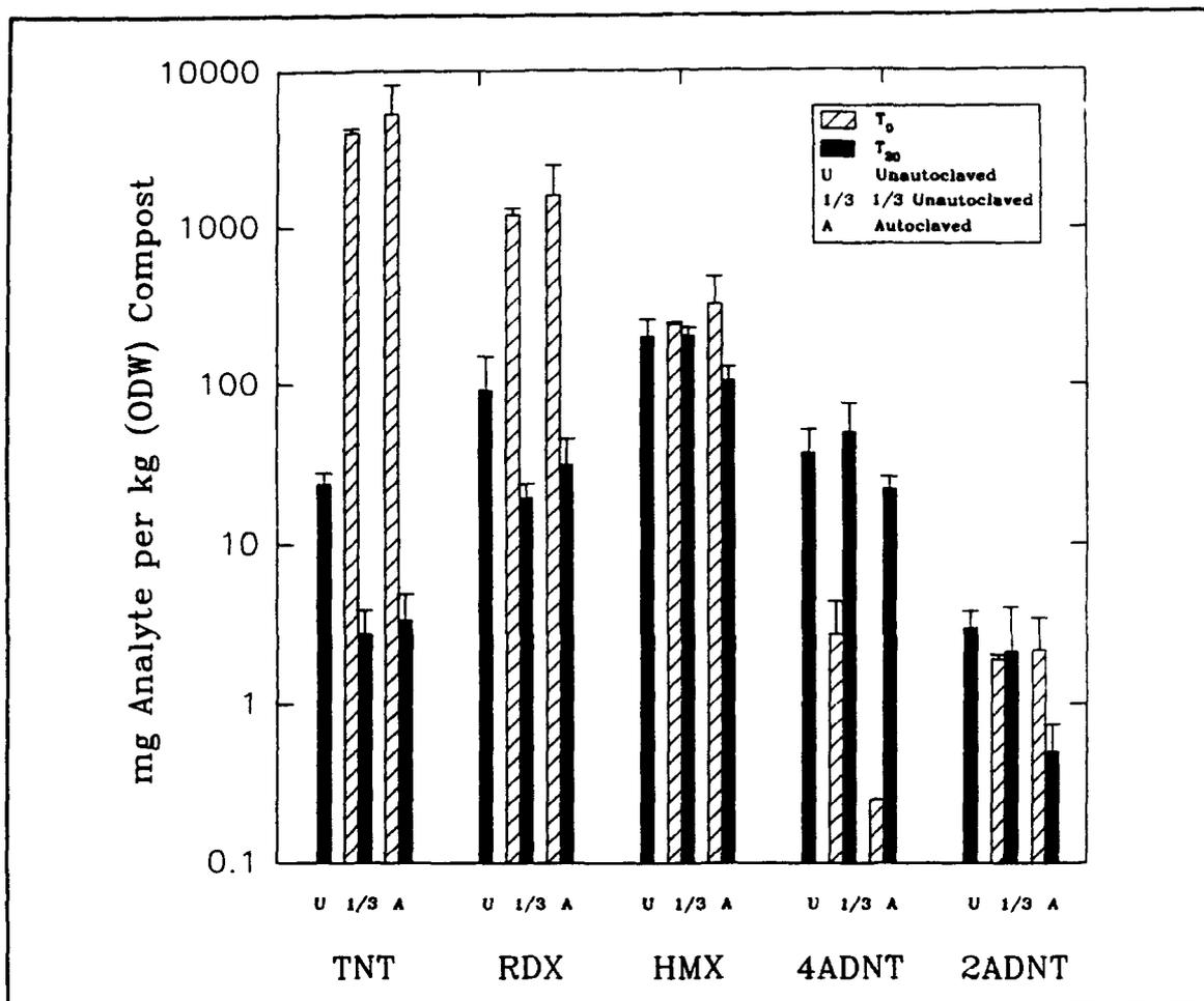
Figure 20. Results of HPLC/UV analysis of composted Umatilla soil from Experiment V at  $T_0$  and  $T_{20}$ . Means of two replicates are shown with standard error bars. The  $T_0$  unautoclaved sample was lost
