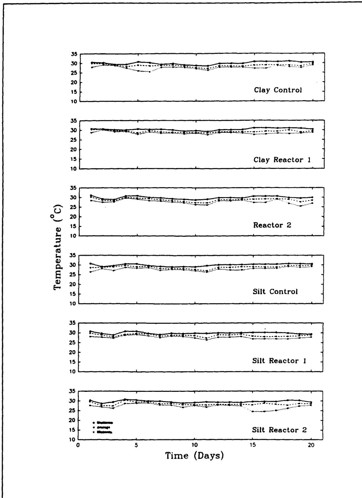
Figure 10. Mean daily maximum, average, and minimum temperatures in composted clay and silt reactors from Experiment II. Each datum point represents average of 30-min readings recorded in each 24-hr period. Controls received no TNT
