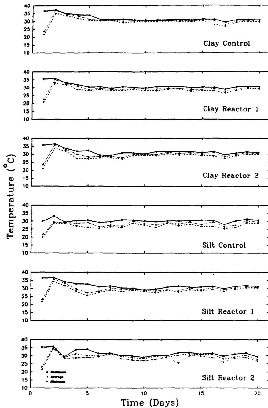
Figure 12. Mean daily maximum, average, and minimum temperatures in composted clay and silt reactors from Experiment III. Each datum point represents average of 30-min readings recorded in each 24-hr period. Controls received no TNT
