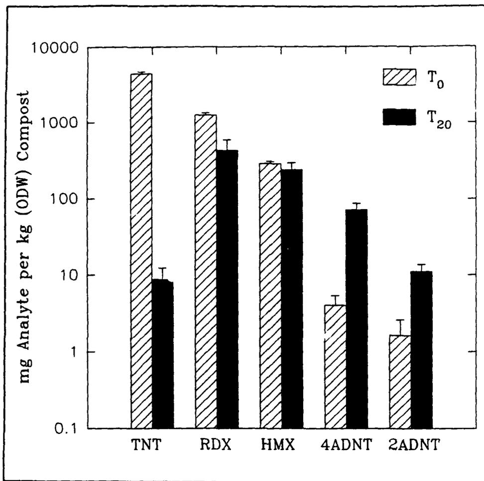
Figure 25. Results of HPLC/UV analysis of composted Umatilla soil at T<sub>0</sub> and T<sub>20</sub> in Experiment VI. Means for all six reactors are shown with standard error bars
