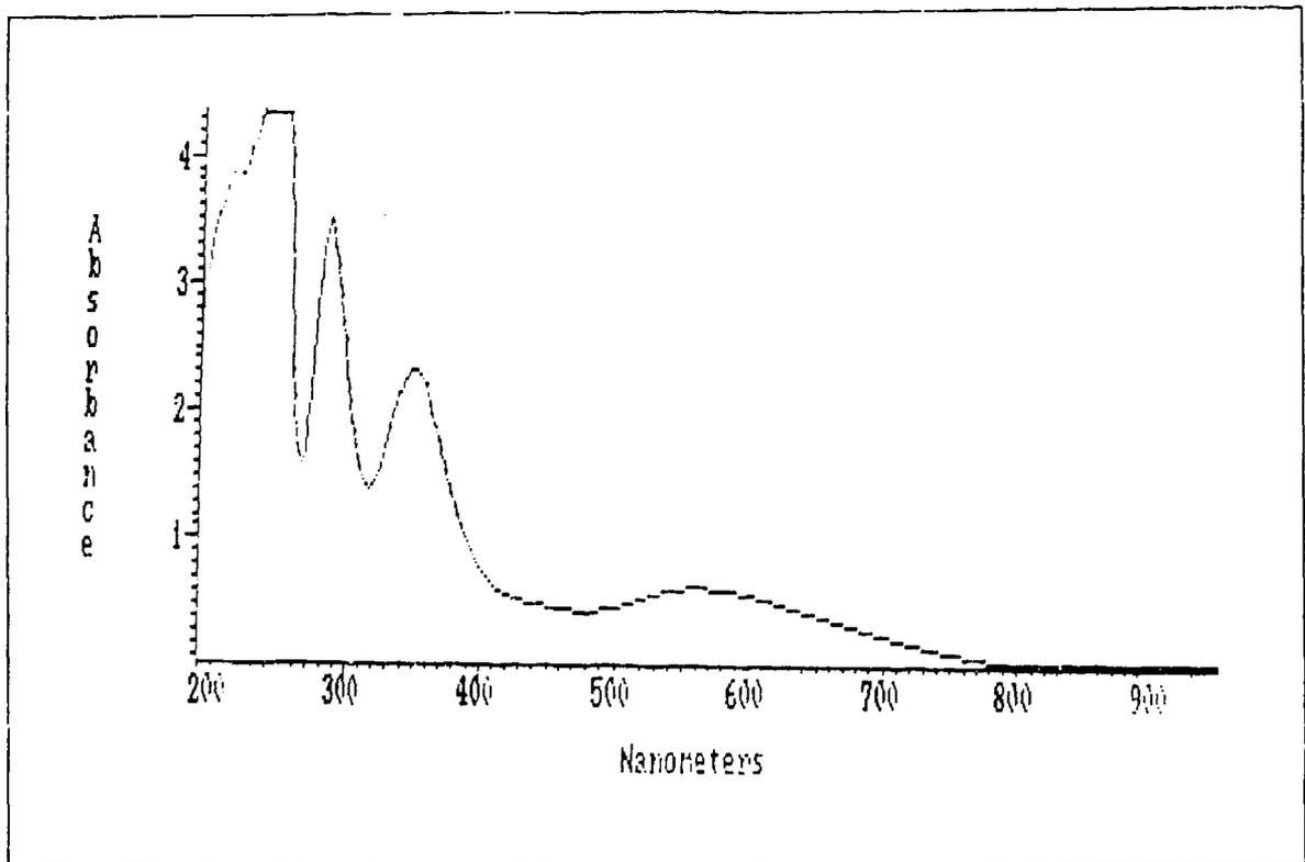
Figure B3. Absorbance of H<sub>2</sub>O<sub>2</sub>, KI, and starch solution:
