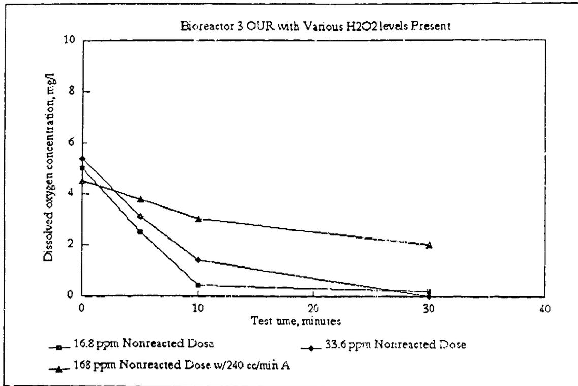
Figure 13. Evaluation of applied residual H<sub>2</sub>O<sub>2</sub> dose on OUR
