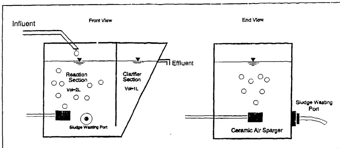
Figure 3. Bench-scale chemostat
