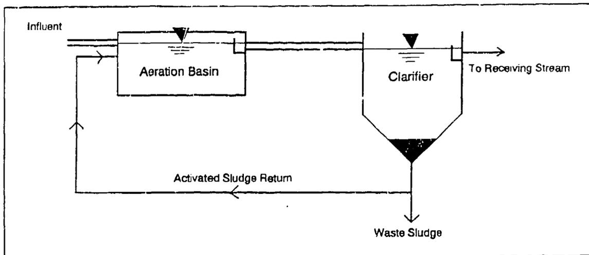
Figure 1. Schematic of a typical activated sludge system
