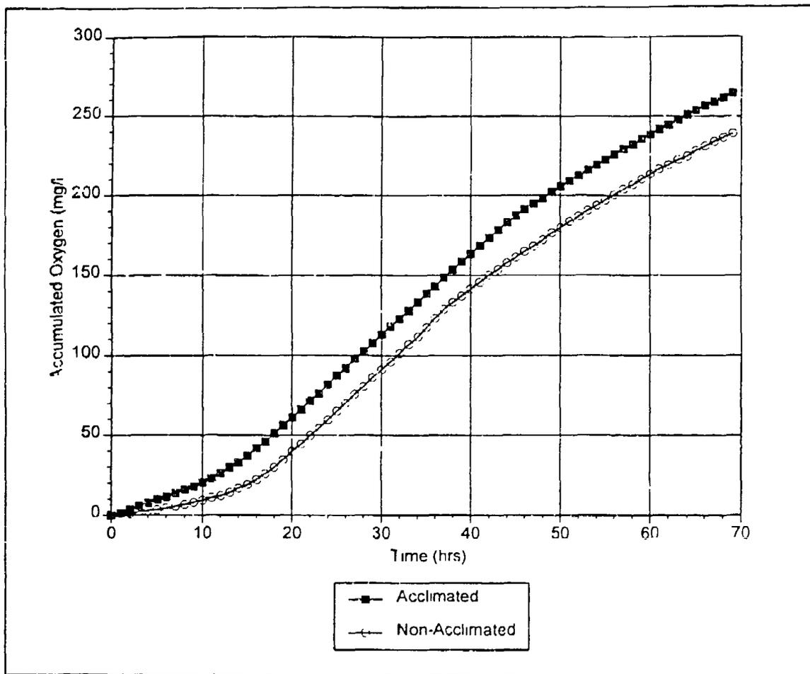
Figure 10. Comparison of acclimated versus unacclimated biomass toward  $H_2O_2$  usage
