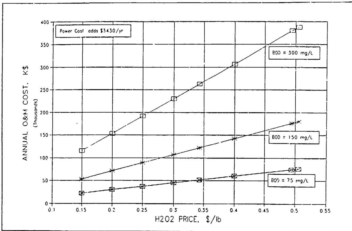
Figure 36 Cost analysis of hydrogen peroxide dosing
