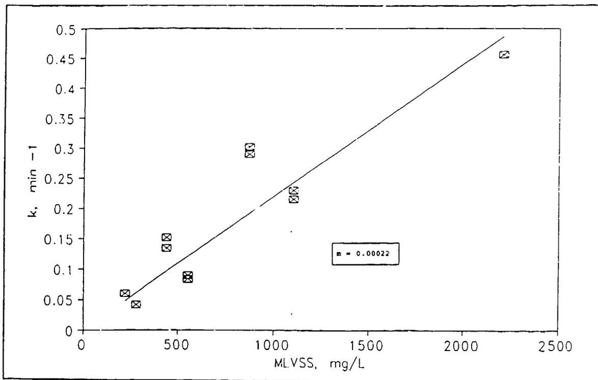
Figure 30. First order reaction rates for 100-mg/l  $H_2O_2$  versus MLVSS
