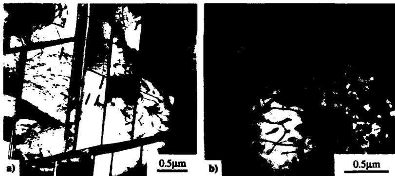
Figure 1 TEM micrographs of the microstructures after creep testing at 760°C: a) the alloy, and b) the composite.
