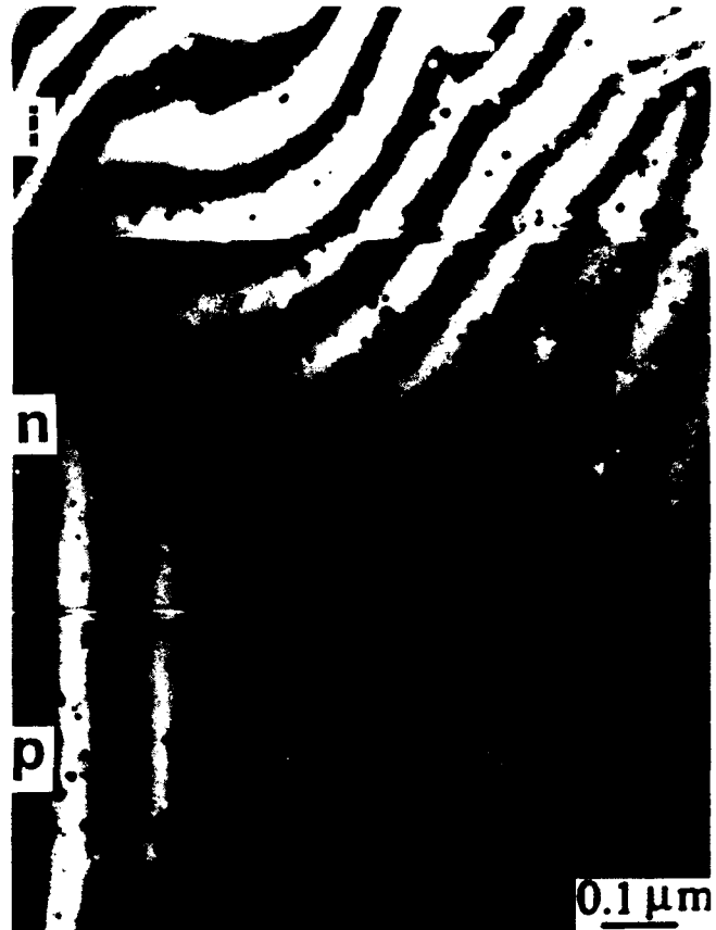
Fig. 3. (111) dark field image of the p-n-i layer structure annealed at 700°C for 10 h.
