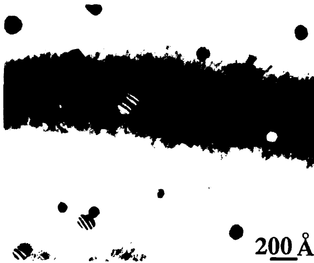
Fig. 2. (111) dark field image of the p-type region in the sample annealed at 700°C for 3 h.
