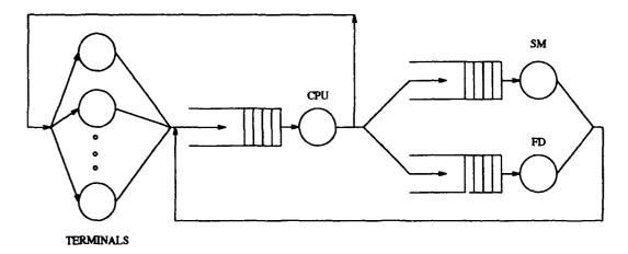
Figure 2: Multiprogrammed Queueing Network Model
