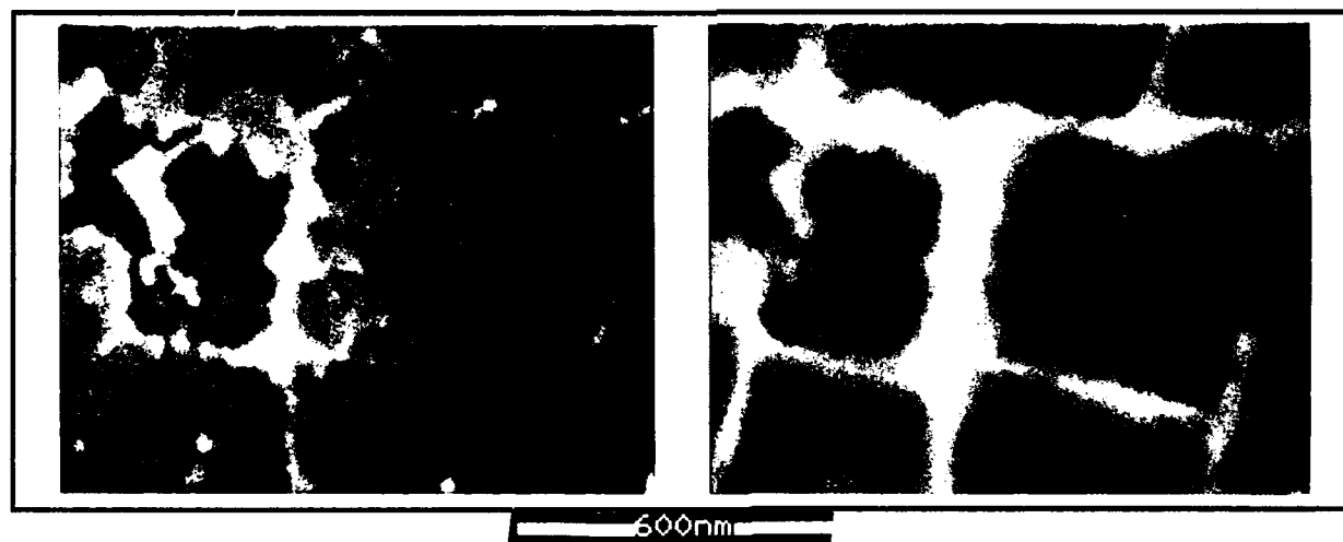
Figure 5. Inter-phase fracture in PWA 1484 from a fatigue test in 5000 psi gaseous hydrogen simulating a rocket environment. The fracture is imaged in secondary emission (left) for topographical contrast and suggests octahedral fracture of the \gamma-\gamma' matrix surrounding the cubic precipitates. The backscattered electron image (right) delineates the areas of the \gamma matrix on the fracture surface.
