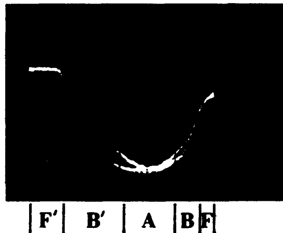
Fig. 3. Birefringence as a function of the polarization. The horizontal and vertical scales are 10 \mu\text{C}/\text{cm}^2 per division and -0.7 \times 10^{-2} , respectively.
