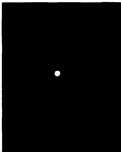
Figure 5. Selected Area Electron Diffraction (SAED) Pattern of Cd_{0.96}Zn_{0.04}Te crystal.
