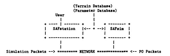
Modelling parameters used in the construction of the ModSAF system are contained in the Parameter Database (DB). Use of this set of parameter files allows modification of the ModSAF system without further computer programming. Both the SAFstation and the SAFsim have access to a Terrain DB.
