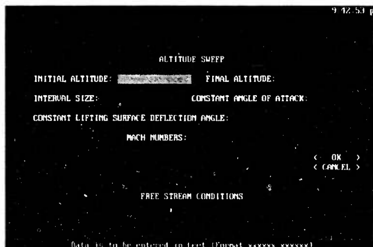
FIGURE 27. FREE-STREAM CONDITIONS-ALTITUDE SWEEP DATA ENTRY SCREEN
