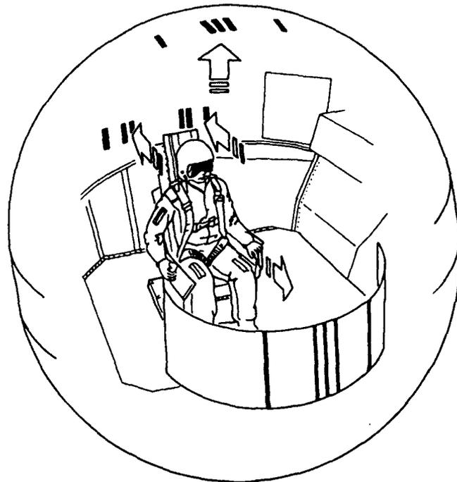
Fig. 1. Dynamic Environment Simulator gondola configuration.
