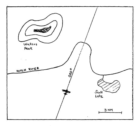
Figure 1. A fictitious map used to illustrate the method of navigation by pilotage.
