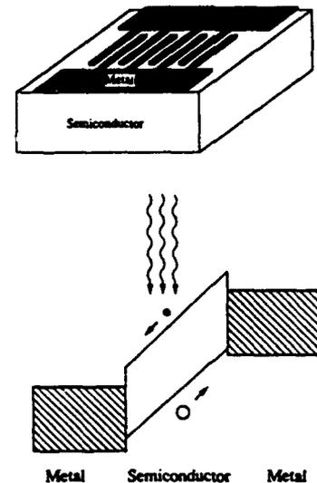
Fig. 1. Schematic view and band diagram of a MSM photodetector.
