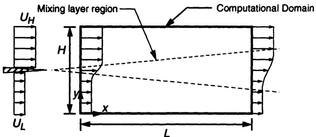
**FIG. 1.** Coordinate system and computational domain for the spatially-developing mixing layer.
