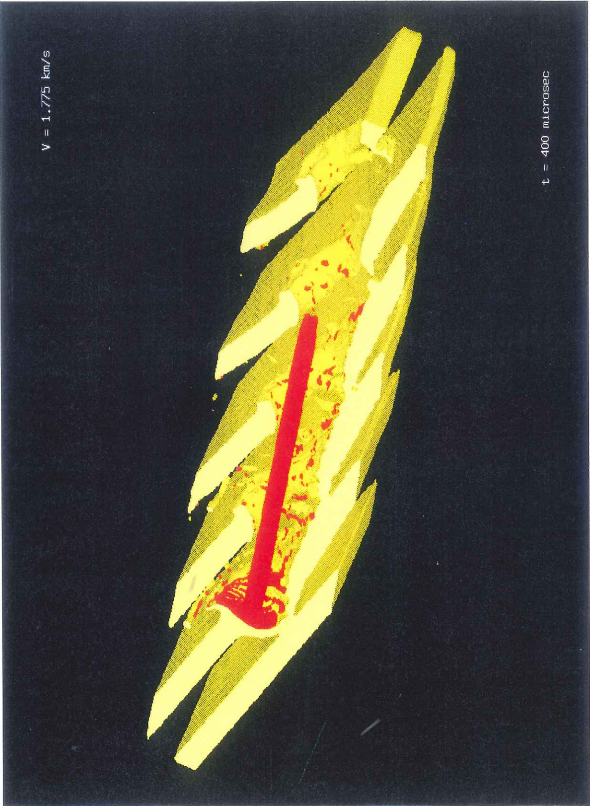
Figure 36. 3-D views of projectile-target interaction: V_p = 1.775 km/s. c) t = 400 \mu s
