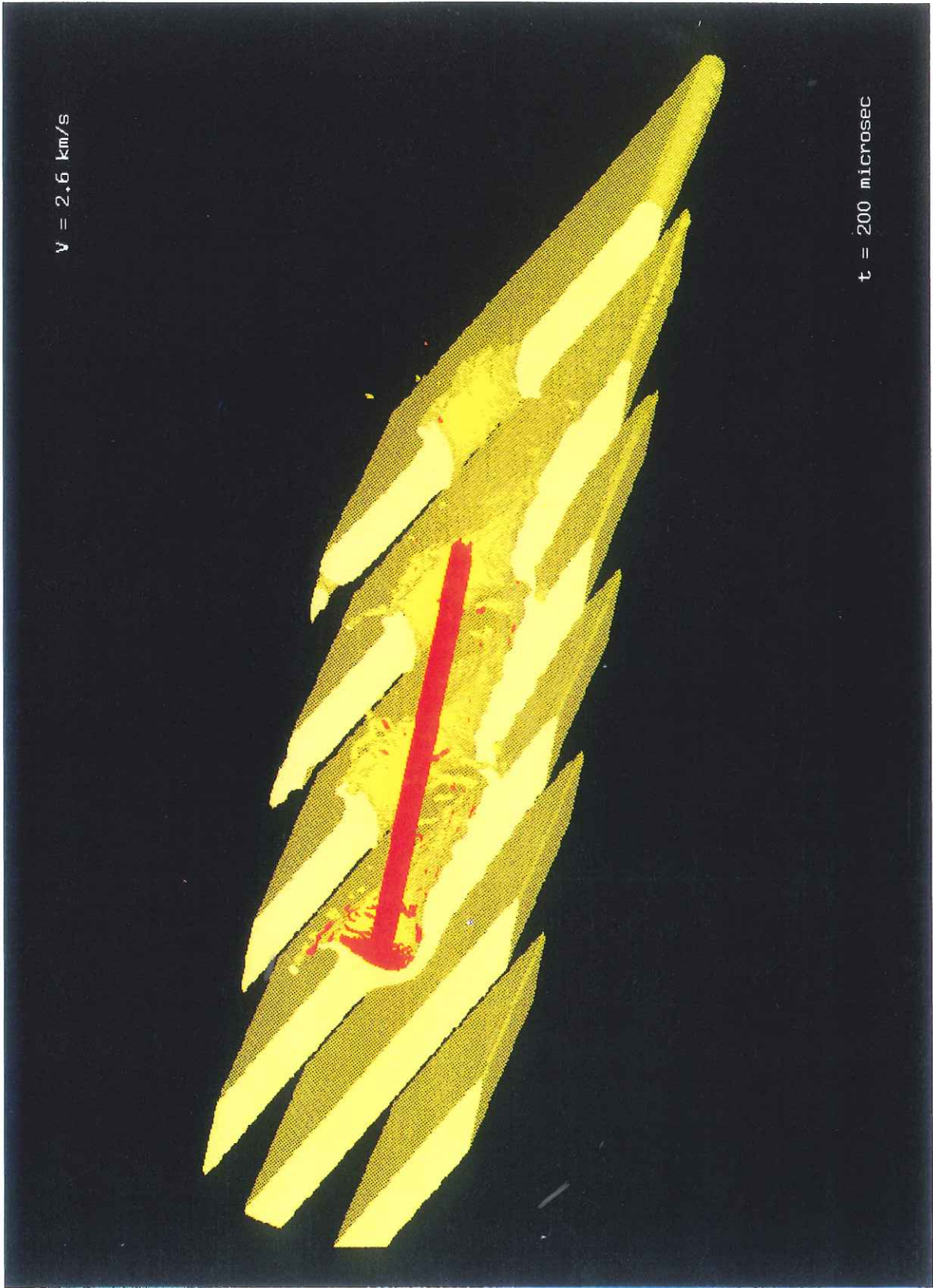
Figure 37. 3-D views of projectile-target interaction: V_p = 2.600 \text{ km/s} . a) t = 200 \mu\text{s}
