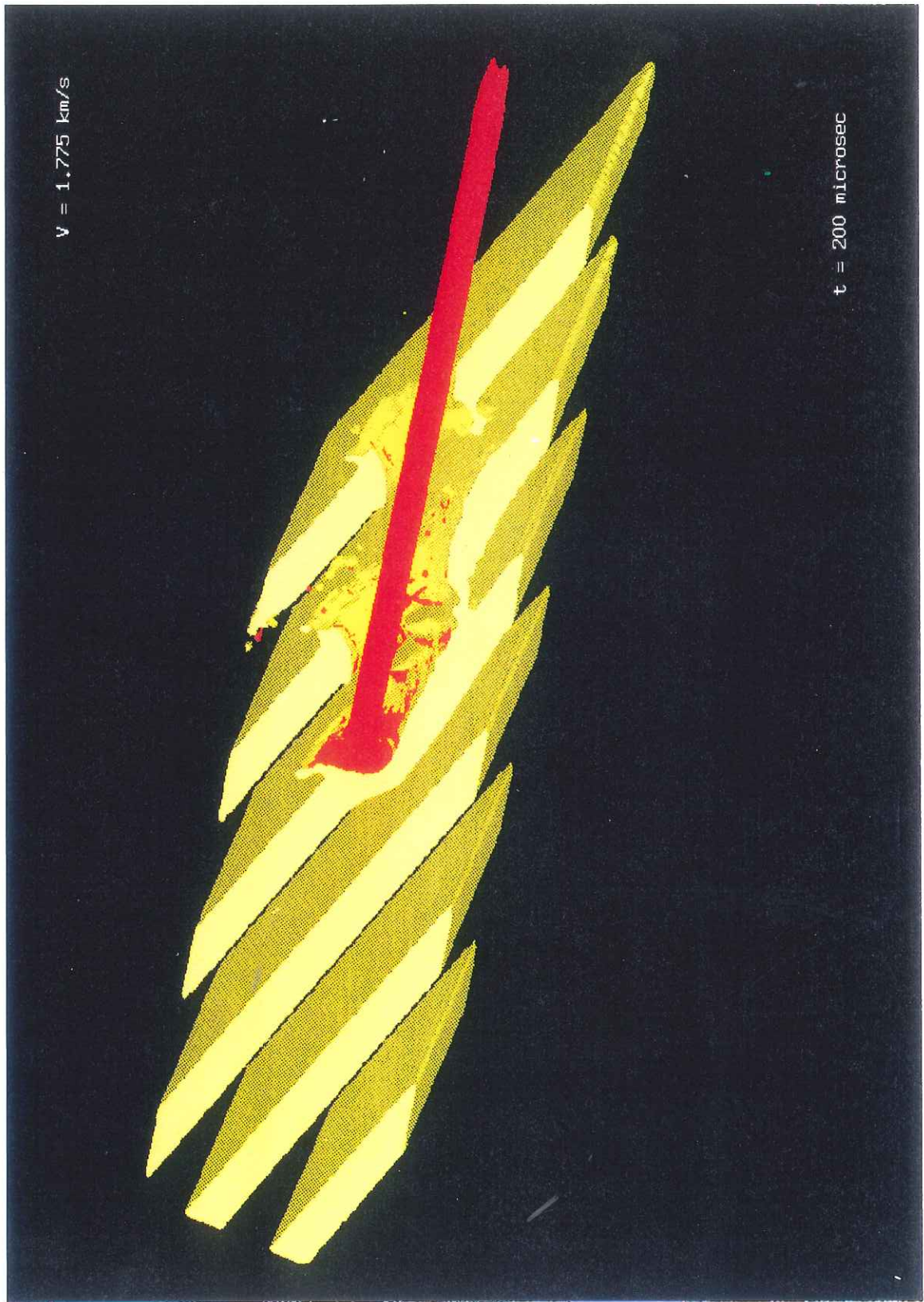
Figure 36. 3-D views of projectile-target interaction: V_p = 1.775 \text{ km/s} . b) t = 200 \mu\text{s}
