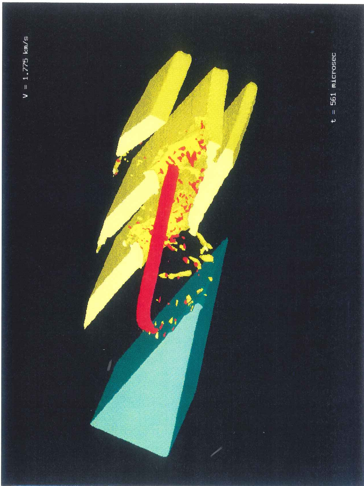
Figure 36. 3-D views of projectile-target interaction: V_p = 1.775 \text{ km/s} . e) t = 561 \mu\text{s} (enlarged view)
