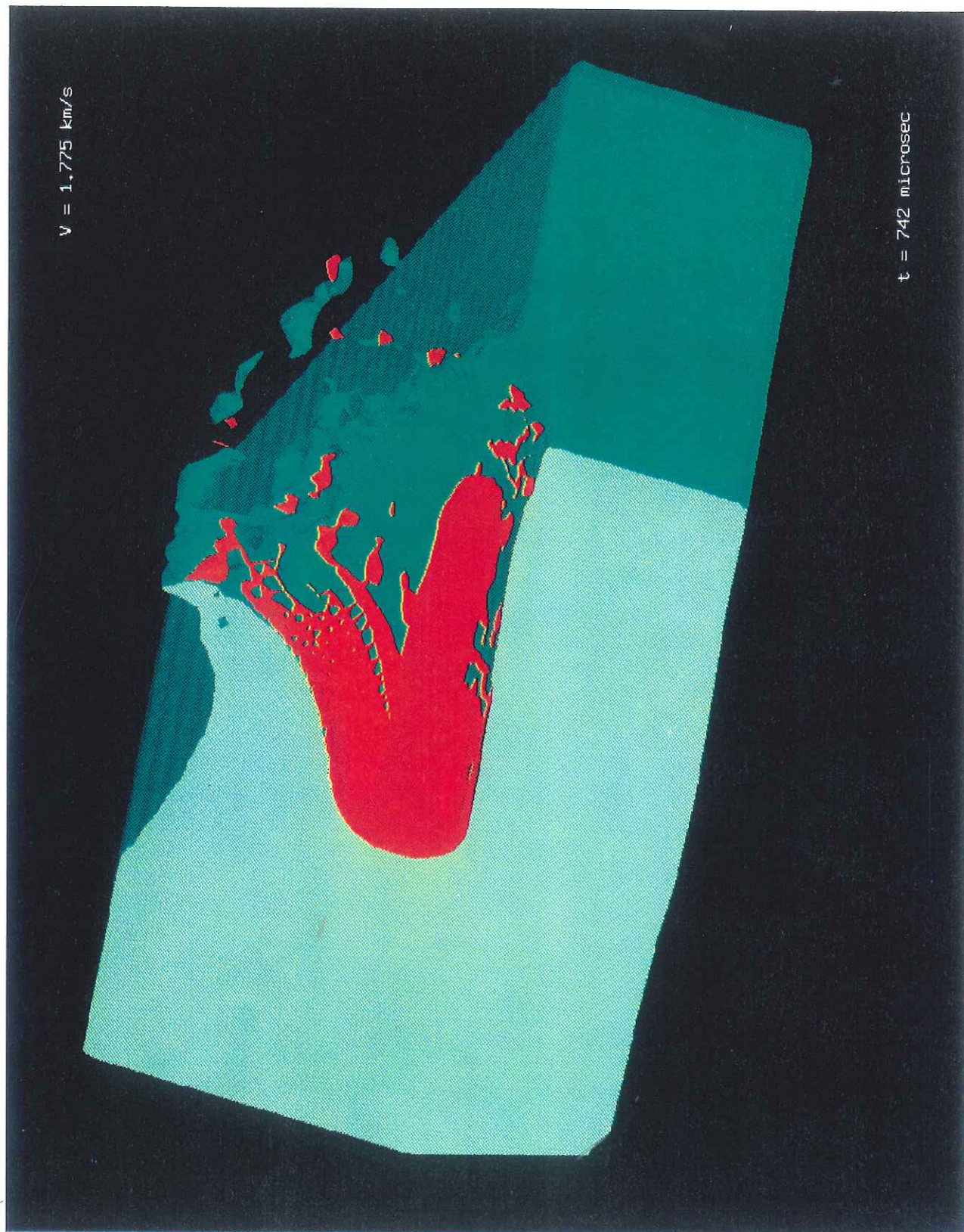
Figure 36. 3-D views of projectile-target interaction: V_p = 1.775 \text{ km/s} . f) t = 742 \mu\text{s}
