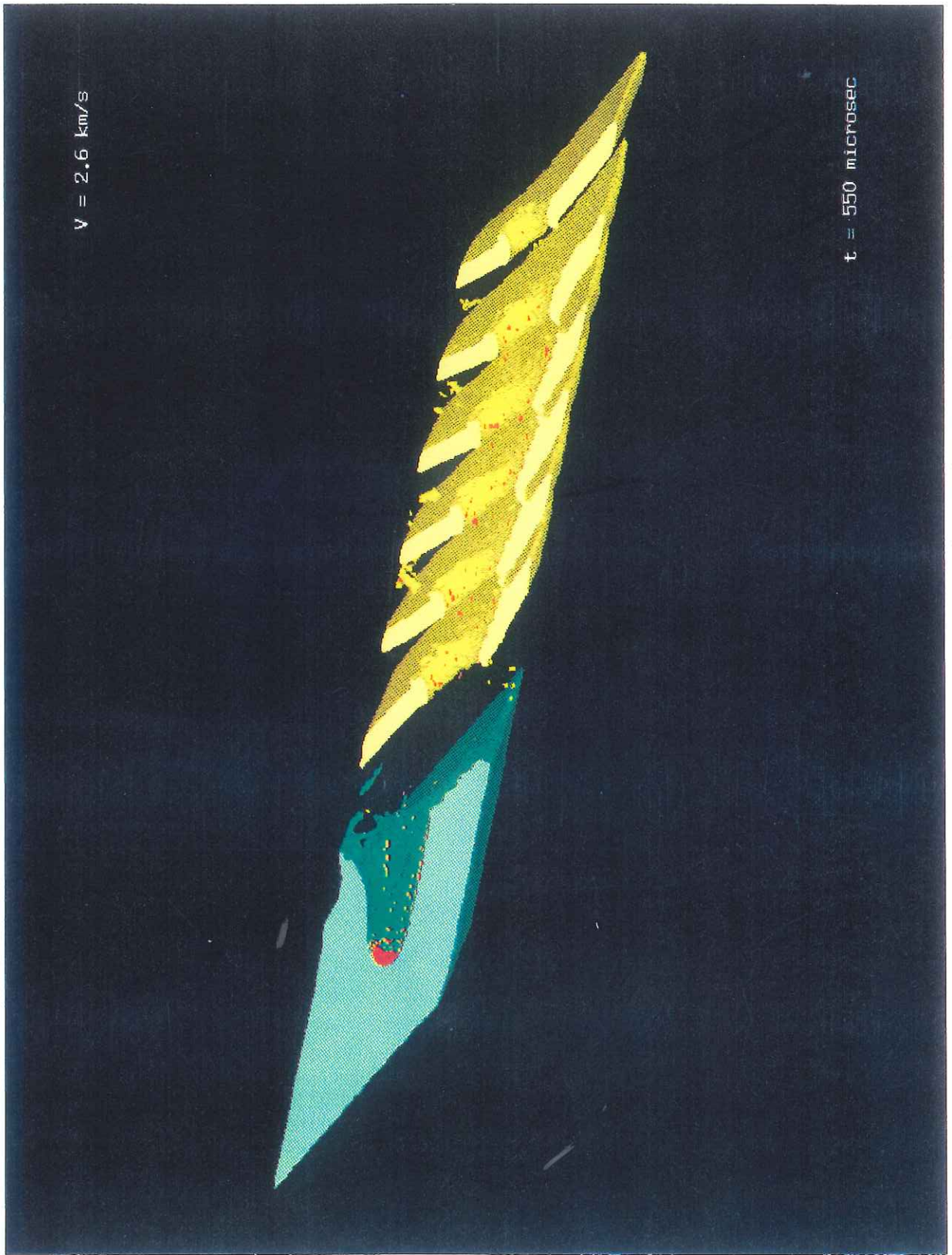
Figure 37. 3-D views of projectile-target interaction: V_p = 2.600 \text{ km/s} . c) t = 550 \mu\text{s}
