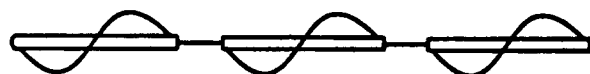
Figure 2. A segmented screw that has a helix interrupted at regular intervals along the linear backbone.
