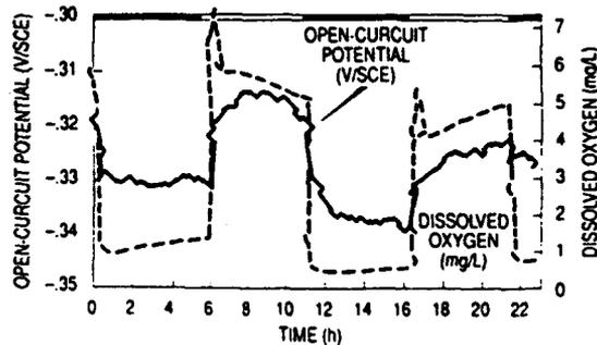
FIG. 2—Open-circuit potential and dissolved oxygen oscillations associated with an *Anabena sp.* biofilm under a 6h light/dark regime. Light period denoted by white slot, dark period denoted by black slot [8].
