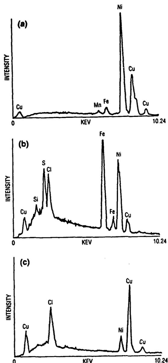
FIG. 8—EDS spectra for nickel alloy Monel 400 before and after exposure to estuarine water [30]: (a) = unexposed, (b) = exposed for 6 months, showing accumulations of Si, S, and Cl with increased Fe and Ni, and (c) = residual metal in base of pit showing Ni depletion and Cu enrichment.
