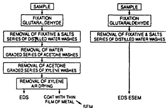
FIG. 7—Flow chart comparing sample preparation for SEM and ESEM.
