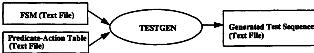
Figure 29 : The General Structure of TESTGEN Program
