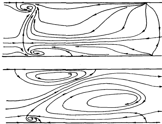
Fig.11 The incipient and developed asymmetry in the surface streamline pattern
