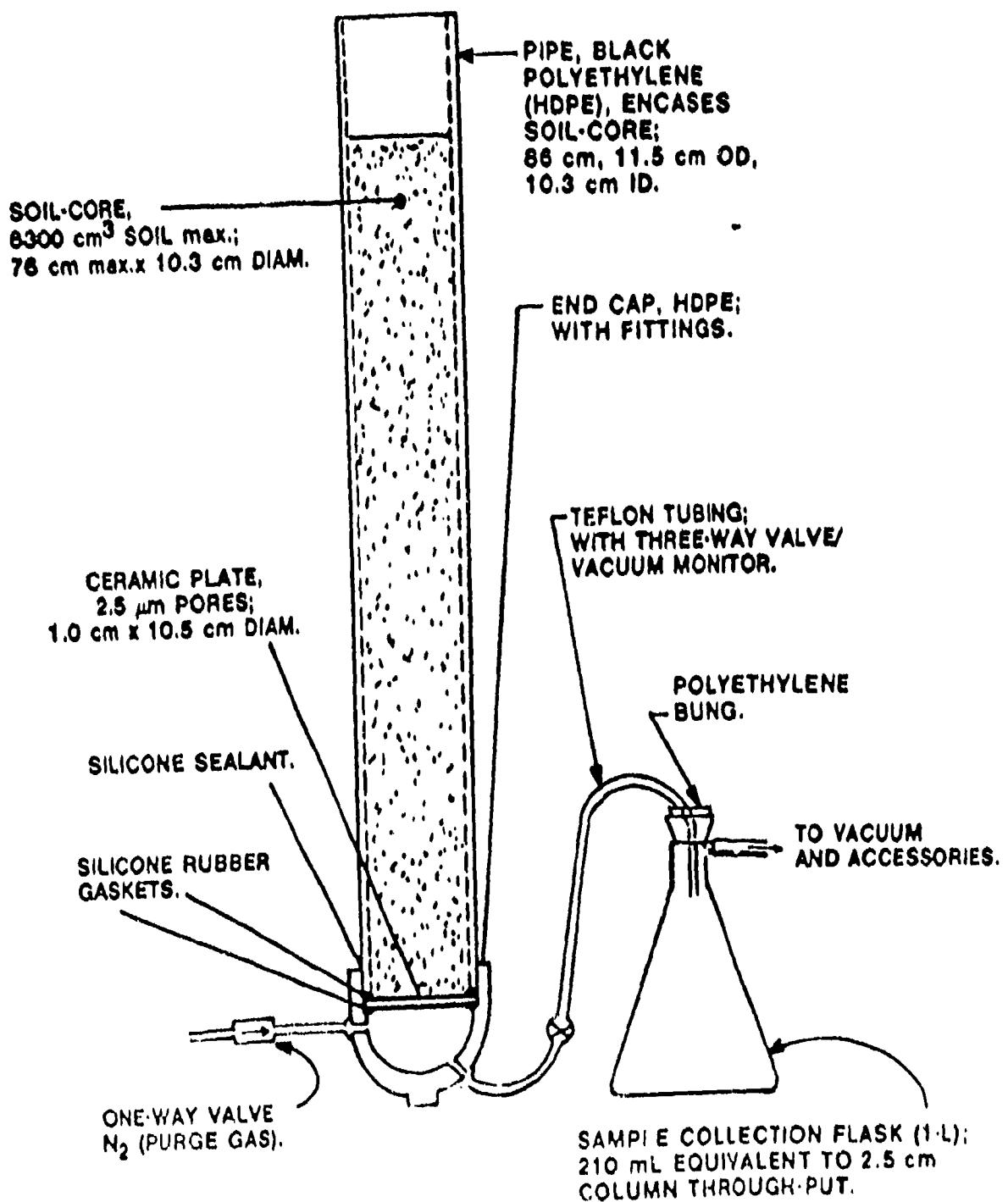
FIGURE 2.3 CROSS-SECTION OF CESMU SYSTEM SHOWING ONE SOIL-CORE COLUMN AND VACUUM SYSTEM.
