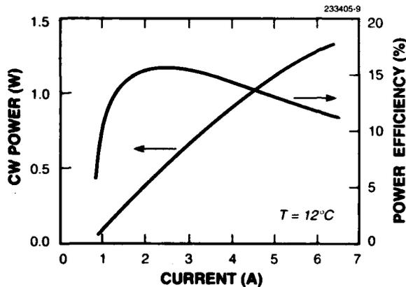
Figure 3-3. Output power vs current for CW operation of 300- $\mu\text{m}$ -wide by 1000- $\mu\text{m}$ -long GaInAsSb/AlGaAsSb quantum-well laser.
