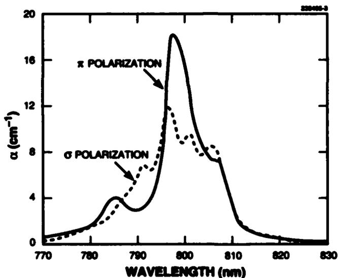
Figure 2-1. Polarization-resolved absorption spectra of Tm:YVO<sub>4</sub> with Tm concentration of 5 at.%.
