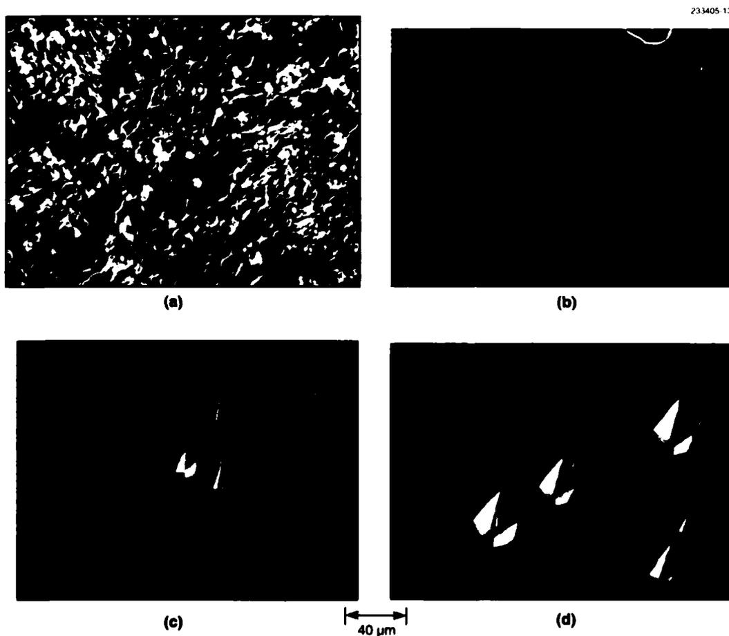
Figure 3-5. Surface morphology of GaSb layers grown on GaAs substrates at 600°C and with V/III ratios of (a) 0.7, (b) 0.8, (c) 0.9, and (d) 1.0.
