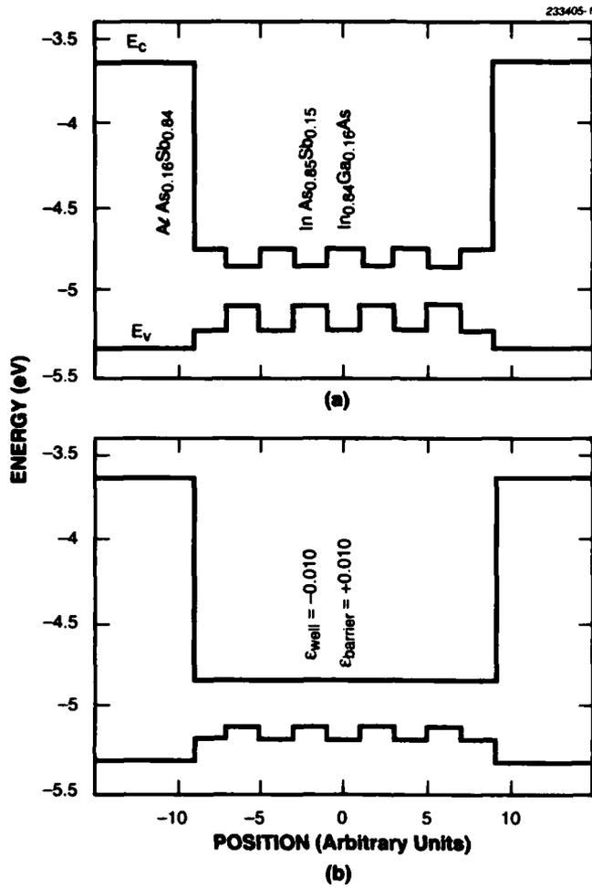
Figure 1-1. Flat band diagram of  $\text{InAs}_{0.85}\text{Sb}_{0.15}/\text{In}_{0.84}\text{Ga}_{0.16}\text{As}$  multiple-quantum-well (MQW) heterostructure on  $\text{InAs}$  substrate (a) without and (b) with strain-induced bandedge shifts.
