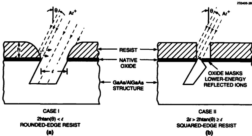
Figure 5-3. Schematic diagrams showing effect of resist geometry on  $Cl_2$ -IBAE etching of small structures. In (a) reflected ions do not significantly contribute to the sidewall slope, as compared to (b) where they aid in forming a structure useful in vacuum-microelectronics applications.
