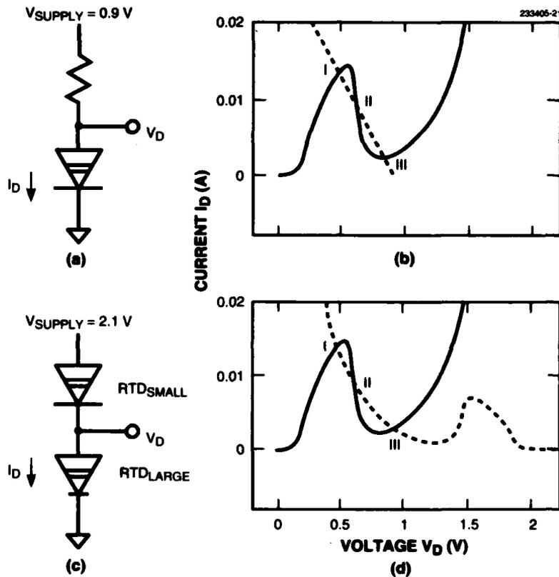
Figure 4-5. Resonant-tunneling diode (RTD) circuits demonstrating bistable operation. (a) Diagram and (b) current-voltage ( $I$ - $V$ ) characteristic for RTD with resistive load. (c) Diagram and (d)  $I$ - $V$  characteristic for RTD with smaller RTD load. In (b) and (d) the dashed lines indicate load lines. For both (b) and (d) the intersections of the load lines with the device characteristics determine the possible operating points (labeled I, II, and III) for the circuits.
