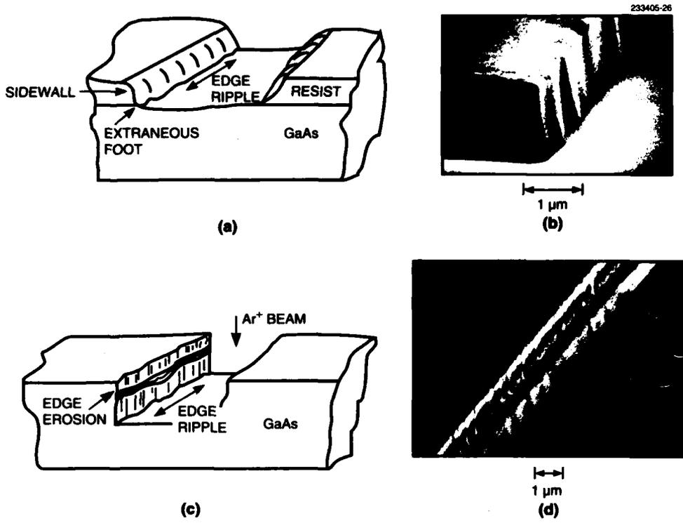
Figure 5-1. Sketches and scanning electron micrographs (SEMs) showing important resist parameters and their effect on the etching process. (a) Diagram and (b) SEM showing resist edge ripple and sloped sidewalls; also seen in (a) is an extraneous foot. (c) Diagram and (d) SEM showing edge erosion and edge ripple produced in the GaAs after etching the structure in (a).
