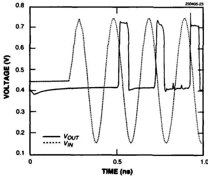
Figure 4-7. Computer simulation of ten-stage bistable transmission-line structure showing pulse shaping. In this simulation  $Z_0 = 50 \Omega$  and  $R_{term} = 50 \Omega$ . The effective propagation velocity is  $8.3 \times 10^9 \text{ cm s}^{-1}$ , the series resistive loss is  $2.4 \times 10^2 \Omega \text{ cm}^{-1}$ , and the length of each segment is 0.2 cm.
