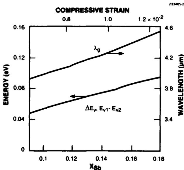
Figure 1-2. Calculated emission wavelength  $\lambda_g$ , valence-band barrier height  $\Delta E_v$ , and valence subband splitting  $E_{v1}-E_{v2}$  for a range of compositions for  $\text{InAs}_{1-x}\text{Sb}_x/\text{In}_{1-y}\text{Ga}_y\text{As}$  MQW heterostructure.
