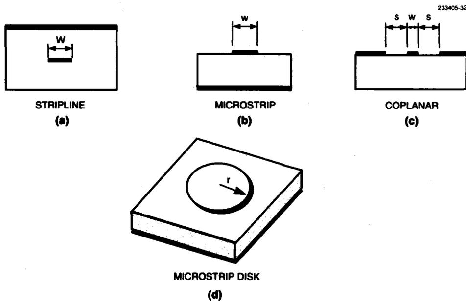
Figure 7-1. Geometries of superconducting resonators: (a)–(c) Cross-sectional views of linear half-wavelength resonators and (d) rotated view of microstrip disk resonator.
