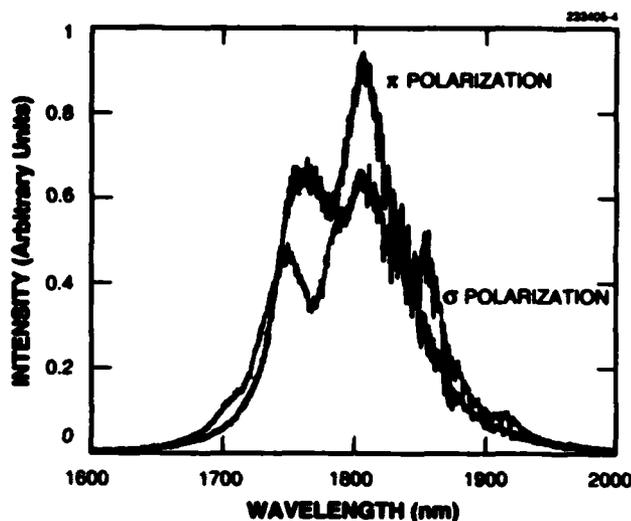
Figure 2-2. Polarization-resolved fluorescence spectra of Tm:YVO<sub>4</sub> with Tm concentration of 5 at.%.
