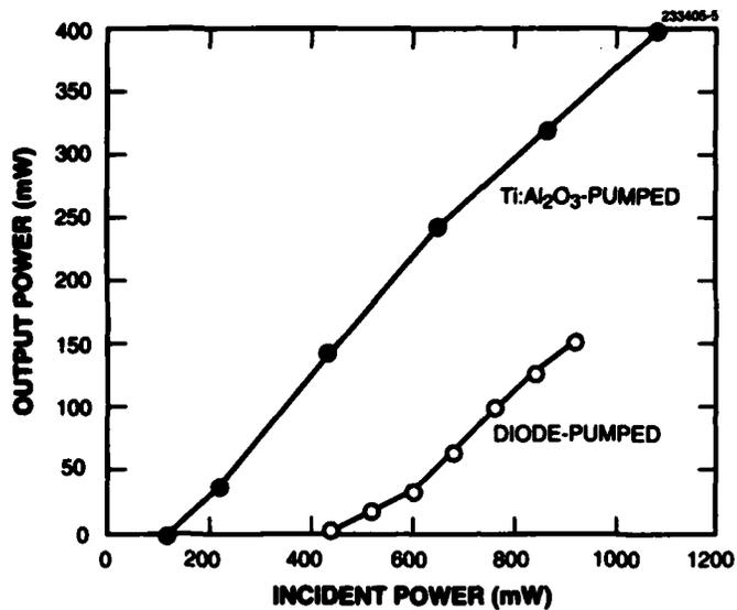
Figure 2-3. Dependence of Tm:YVO<sub>4</sub> microchip laser output power on incident pump power.
