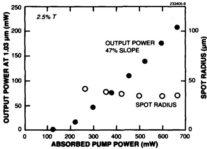
Figure 2-6. Yb:YAG microchip laser output power and cavity mode radius as a function of incident pump power.
