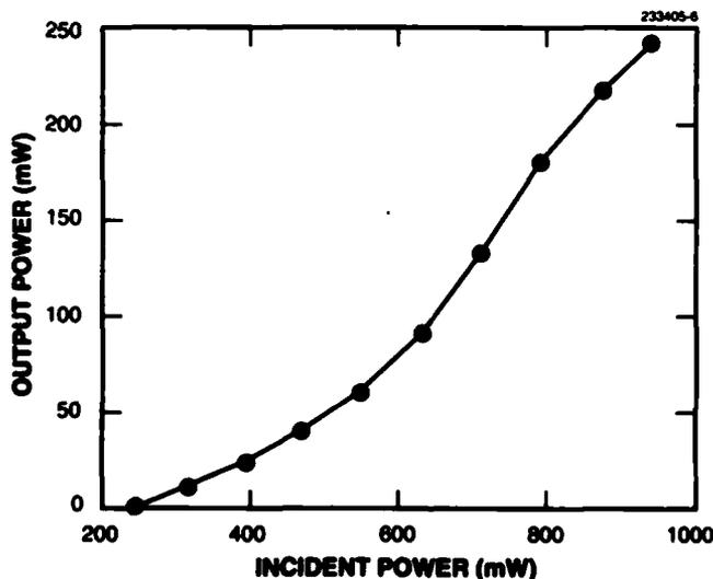
Figure 2-4. Dependence of Nd:YVO<sub>4</sub> microchip laser output power on incident pump power.
