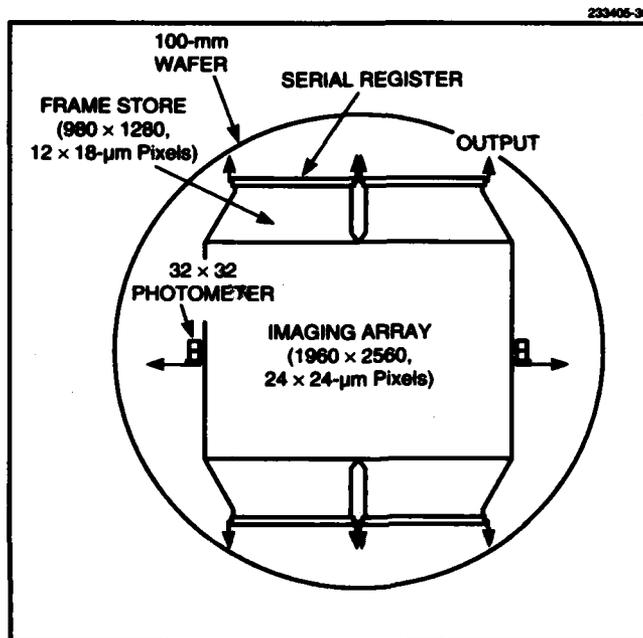
*Figure 6-1. Schematic of 1960 x 2560-pixel frame-transfer charge-coupled device imager. This device fills almost all the usable area of a 100-mm-diam silicon wafer.*
