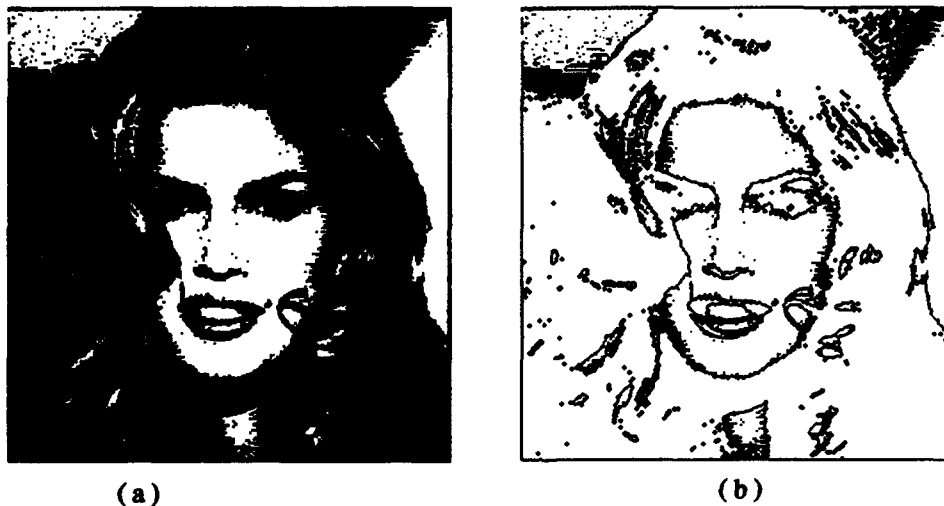
Fig. 3. Image processing. (a) After Averaging Template (b) After Averaging and Edge Detection Templates
