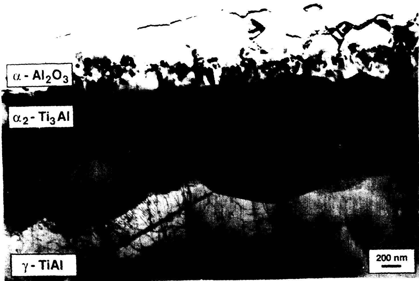
Figure IV.A.1.10 Cross-Section TEM Micrograph of Alumina on Gamma TiAl.
