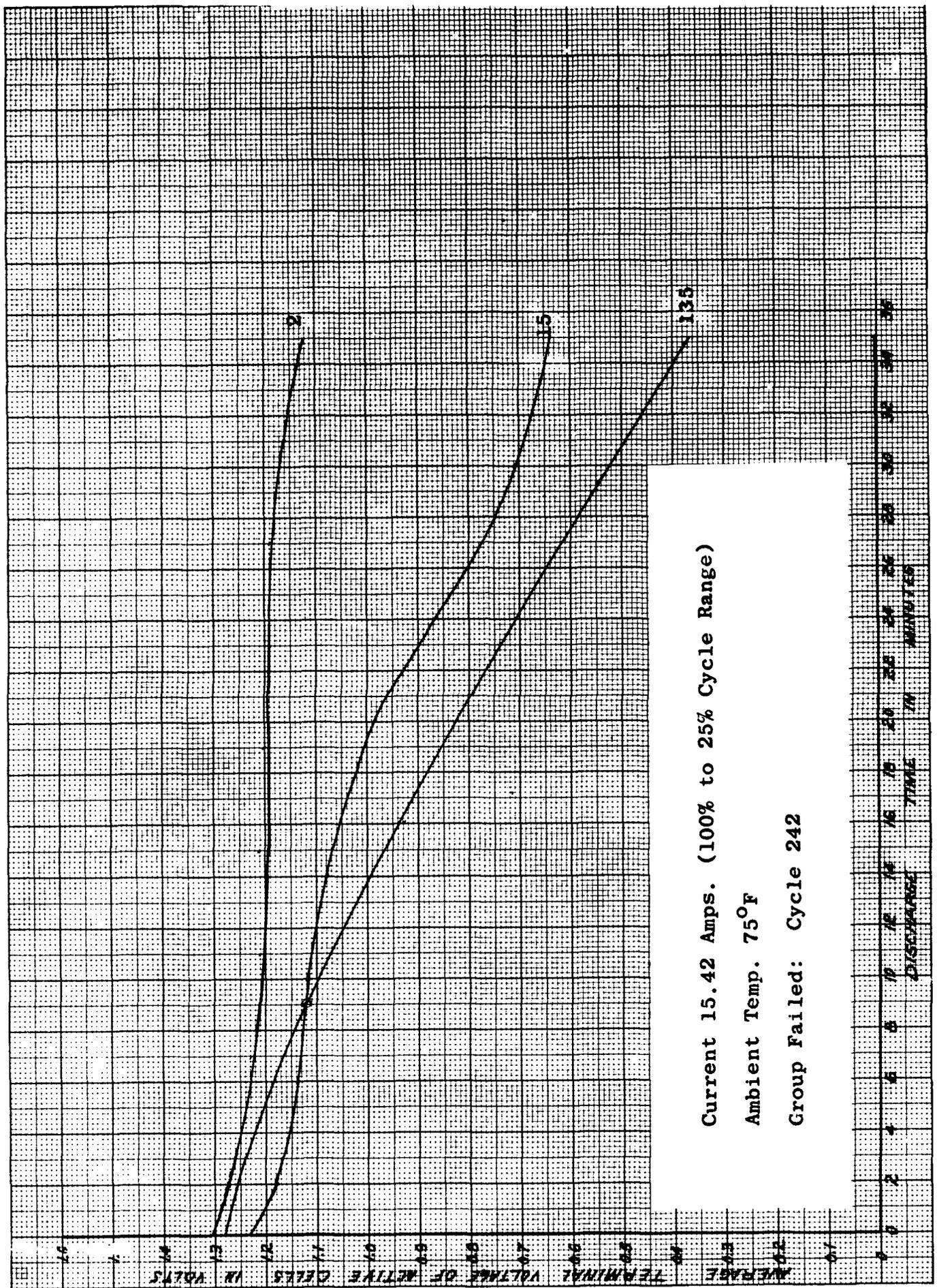
Figure 10 - Discharge Performance - Test Group III
