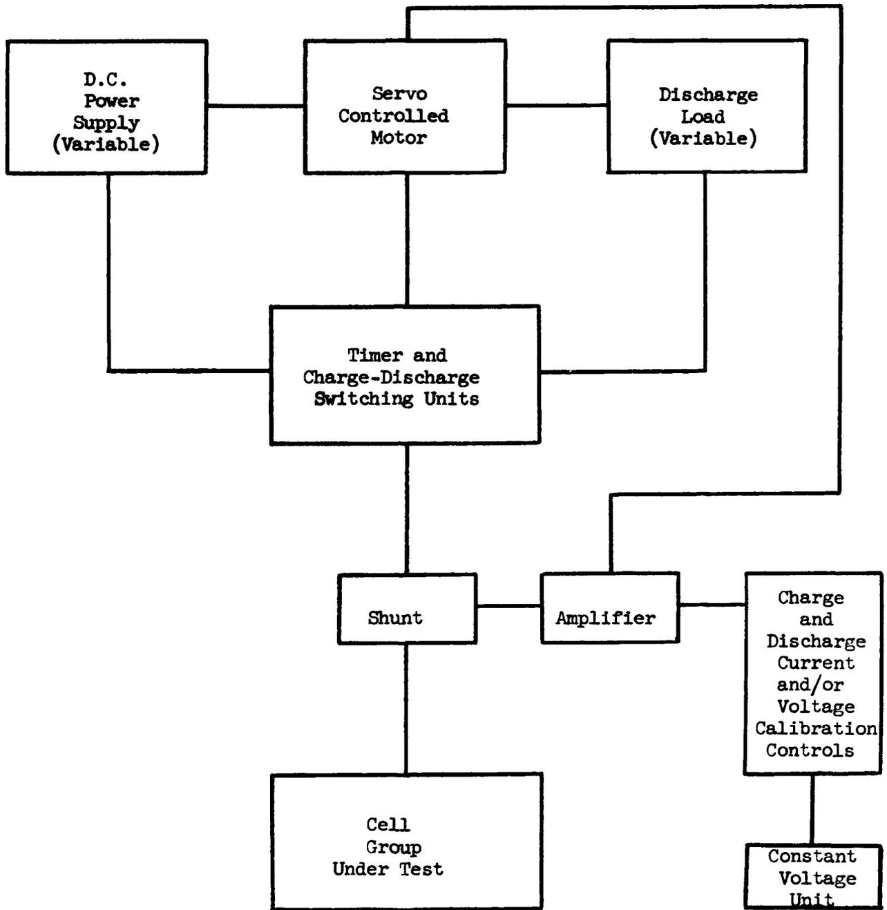
Figure 1 Block Diagram of Charge-Discharge Equipment
