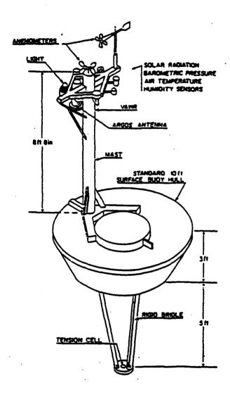
Figure 1. Line drawing of the buoy designed specifically for ERICA.
