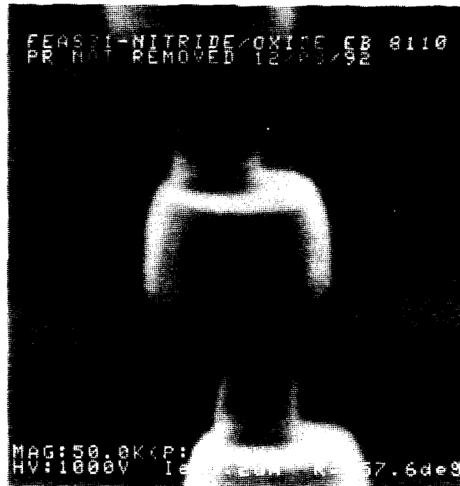
Figure 6: Nitride cap formed postpolishing with photolithographic method.
