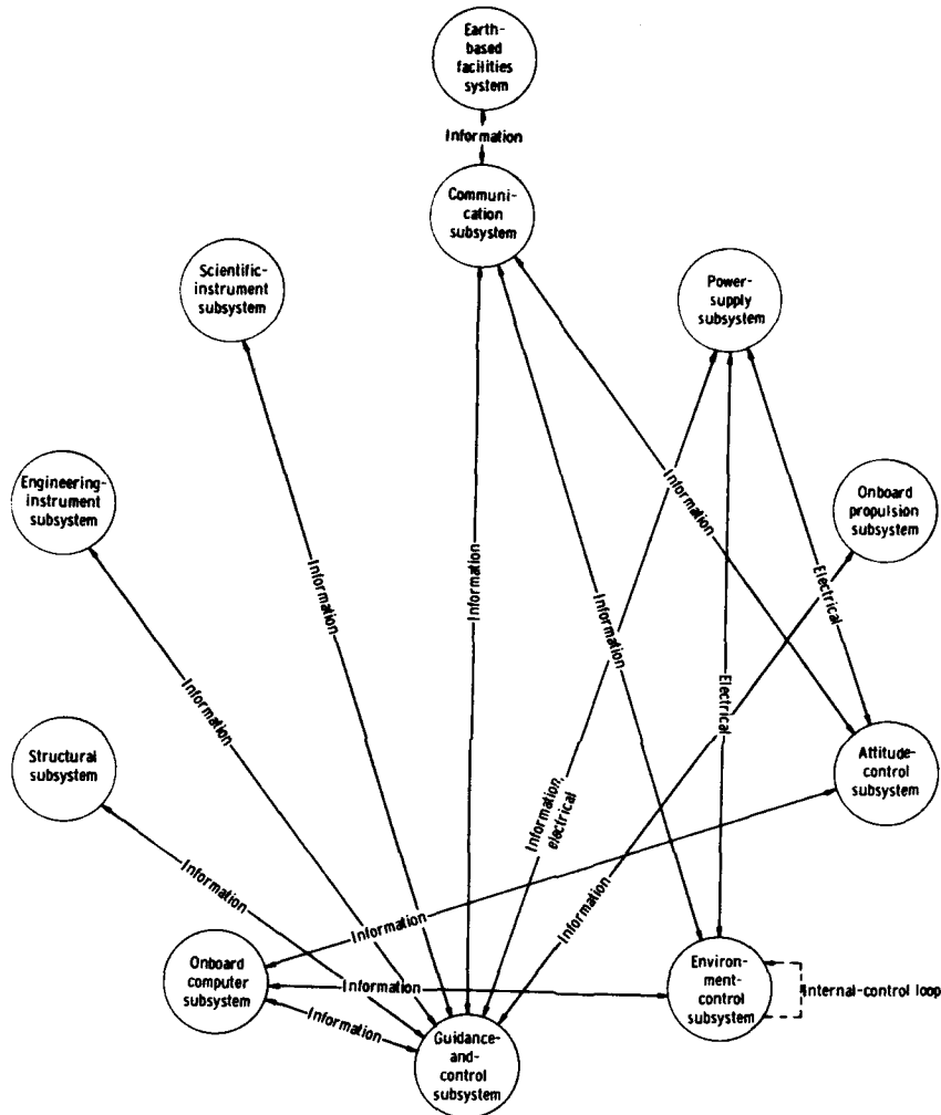
FIGURE 6-2.—Interface diagram showing the more important relationships between the three satellite-control subsystems and the remainder of the spacecraft. The information interface includes the transmission and reception of error and navigational information as well as commands.
