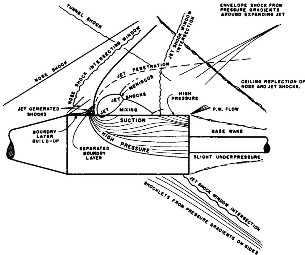
Fig. 18. Flow and pressure regions, from visualization techniques.
