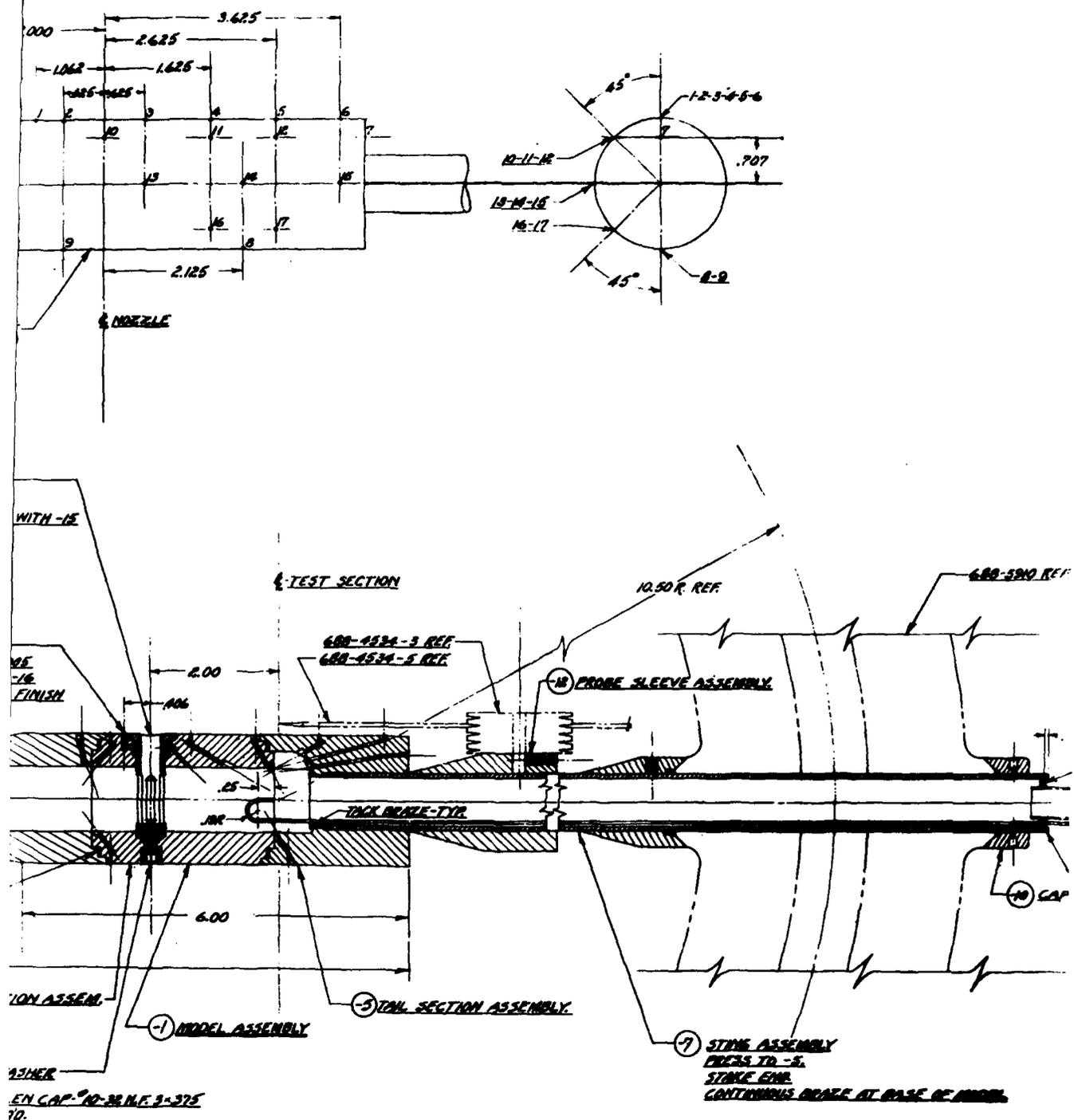
Fig. 2. Pressure orifices and internal model arrangement.
